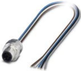
Sensor/Actuator flush-type plug, 5-pos., M12-SPEEDCON, A-coded, front/screw mounting with M16 thread, can be positioned, with 0.5 m TPE litz wire, 5 x 0.25 mm<sup>2</sup>
