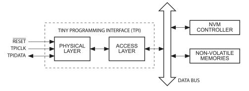
Programming is done via the physical interface. This is a 3-pin interface, which uses the RESET pin as enable, the TPICLK pin as the clock input, and the TPIDATA pin as data input and output.
