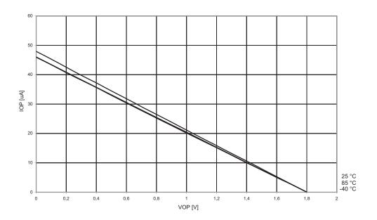
Figure 21-19.I/O Pin Pull-up Resistor Current vs. input Voltage ( $V_{CC} = 2.7V$ )
