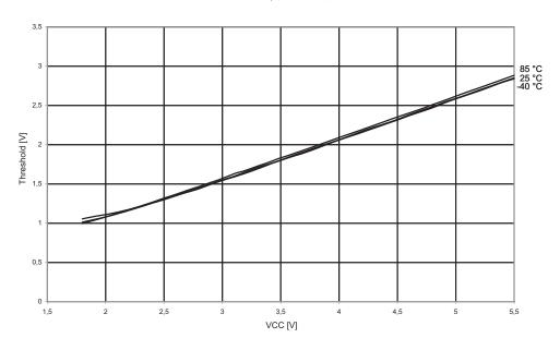
Figure 21-37. $V_{\rm IL}$ : Input Threshold Voltage vs.  $V_{\rm CC}$  (I/O Pin, Read as '0')
