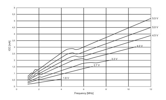
Figure 21-3. Active Supply Current vs. V<sub>CC</sub> (Internal Oscillator, 8 MHz)
