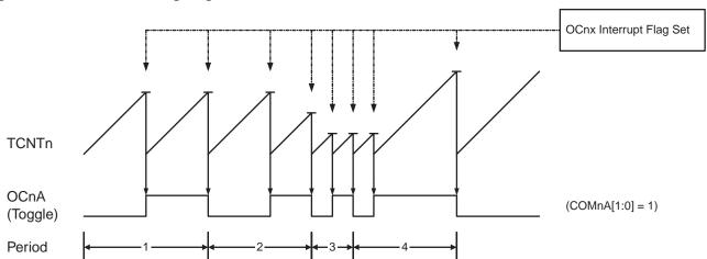
Figure 11-5. CTC Mode, Timing Diagram
