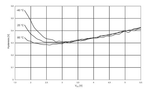
Figure 21-39.V<sub>IH</sub>: Input Threshold Voltage vs. V<sub>CC</sub> (Reset Pin as I/O, Read as '1')
