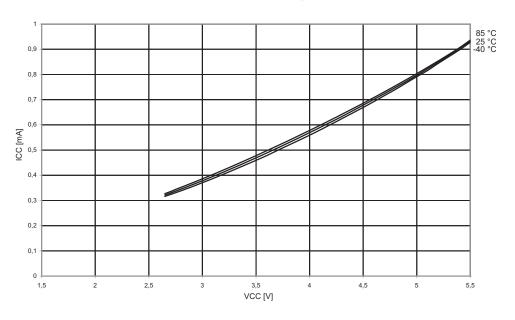
Figure 21-9. Idle Supply Current vs.  $V_{\rm CC}$  (Internal Oscillator, 1 MHz)
