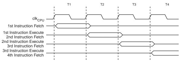
Figure 4-4 shows the parallel instruction fetches and instruction executions enabled by the Harvard architecture and the fast access Register File concept. This is the basic pipelining concept to obtain up to 1 MIPS per MHz with the corresponding unique results for functions per cost, functions per clocks, and functions per power-unit.
