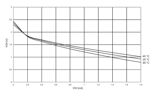
Figure 21-35. $V_{OH}$ : Output Voltage vs. Source Current (Reset Pin as I/O,  $V_{CC}$  = 5V
