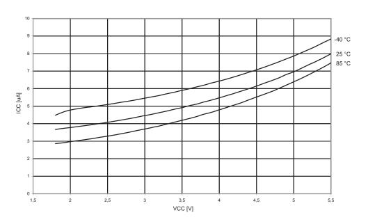
Figure 21-17.Brownout Detector Current vs.  $V_{\rm CC}$
