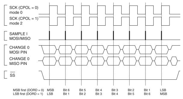
Figure 16-4. SPI Transfer Format with CPHA = 1
