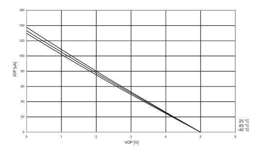
Figure 21-21.Reset Pull-up Resistor Current vs. Reset Pin Voltage ( $V_{CC} = 1.8V$ )
