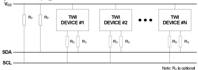
A unique address is assigned to all slave devices connected to the bus, and the master will use this to address a slave and initiate a data transaction. 7-bit or 10-bit addressing can be used.
