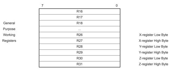
Note: A typical implementation of the AVR register file includes 32 general purpose registers but ATtiny20 implements only 16 registers. For reasons of compatibility the registers are numbered R16:R31 and not R0:R15.
