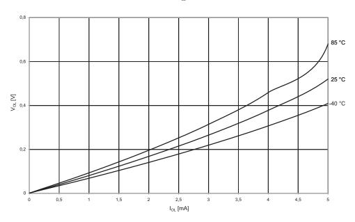
Figure 21-25. $V_{OL}$ : Output Voltage vs. Sink Current (I/O Pin,  $V_{CC}$  = 3V)
