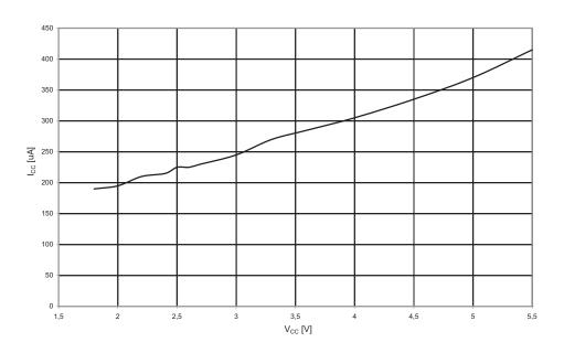
Figure 21-15. Analog Comparator Current vs.  $V_{CC}$
