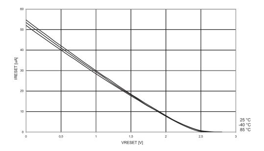
Figure 21-23.Reset Pull-up Resistor Current vs. Reset Pin Voltage (V<sub>CC</sub> = 5V)
