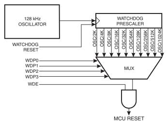
The Watchdog Timer can also be configured to generate an interrupt instead of a reset. This can be very helpful when using the Watchdog to wake-up from Power-down.
