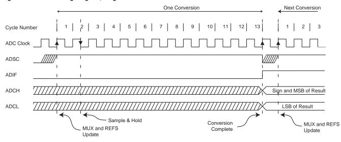
Figure 15-5. ADC Timing Diagram, Single Conversion
