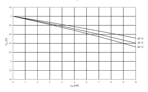
Figure 21-29. $V_{OH}$ : Output Voltage vs. Source Current (I/O Pin,  $V_{CC} = 5V$ )
