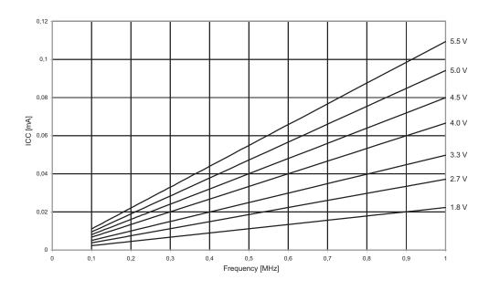
Figure 21-7. Idle Supply Current vs. Frequency (1 - 12 MHz)
