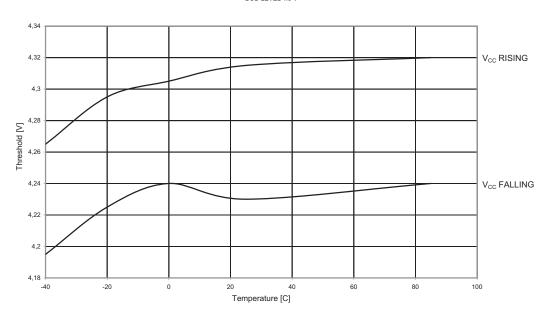
Figure 21-43.BOD Threshold vs Temperature (BODLEVEL is 2.7V)
