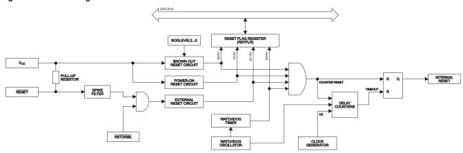
The I/O ports of the AVR are immediately reset to their initial state when a reset source goes active. This does not require any clock source to be running.
