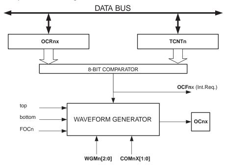
The OCR0x Registers are double buffered when using any of the Pulse Width Modulation (PWM) modes. For the normal and Clear Timer on Compare (CTC) modes of operation, the double buffering is disabled. The double buffering synchronizes the update of the OCR0x Compare Registers to either top or bottom of the counting sequence. The synchronization prevents the occurrence of odd-length, non-symmetrical PWM pulses, thereby making the output glitch-free.
