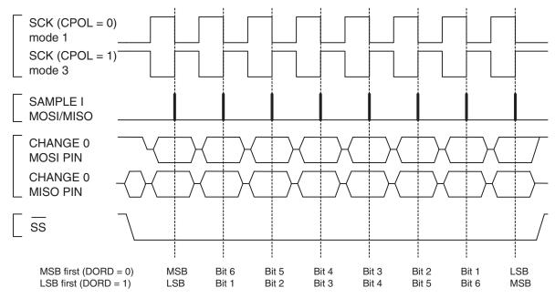
Data bits are shifted out and latched in on opposite edges of the SCK signal, ensuring sufficient time for data signals to stabilize. This is shown in Table 16-2, which is a summary of Table 16-3 and Table 16-4.
