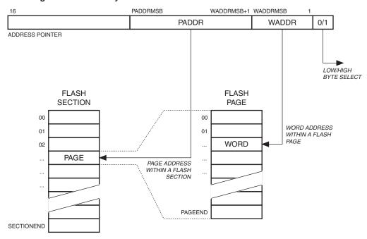
The most significant bits of the data space address select the NVM Lock bits or the Flash section mapped to the data memory. The word address within a page (WADDR) is held by the bits [WADDRMSB:1], and the page address (PADDR) is held by the bits [PADDRMSB:WADDRMSB+1]. Together, PADDR and WADDR form the absolute address of a word in the Flash section.
