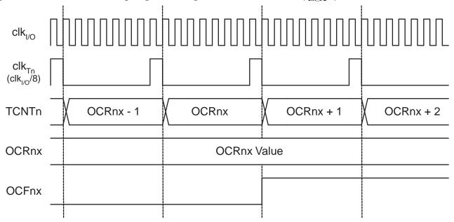
Figure 12-12 shows the count sequence close to TOP in various modes. When using phase and frequency correct PWM mode the OCR1x Register is updated at BOTTOM. The timing diagrams will be the same, but TOP should be replaced by BOTTOM, TOP-1 by BOTTOM+1 and so on. The same renaming applies for modes that set the TOV1 flag at BOTTOM.
