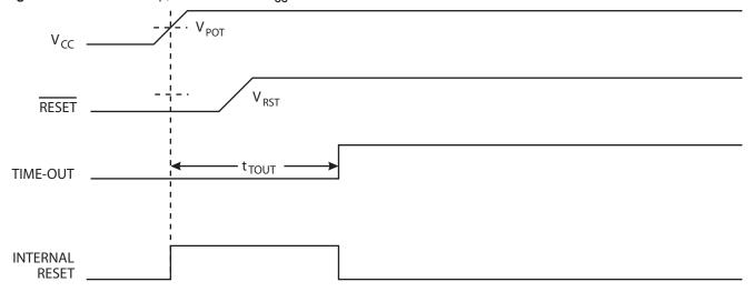
Figure 8-3. MCU Start-up, RESET Extended Externally
