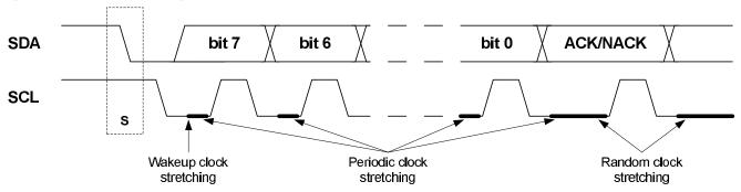
If the device is in a sleep mode and a START condition is detected the clock is stretched during the wake-up period for the device.
