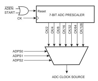
The ADC module contains a prescaler, as illustrated in Figure 15-3 on page 112, which generates an acceptable ADC clock frequency from any CPU frequency above 100 kHz. The prescaling is set by the ADPS bits in ADCSRA. The prescaler starts counting from the moment the ADC is switched on by setting the ADEN bit in ADCSRA. The prescaler keeps running for as long as the ADEN bit is set, and is continuously reset when ADEN is low.
