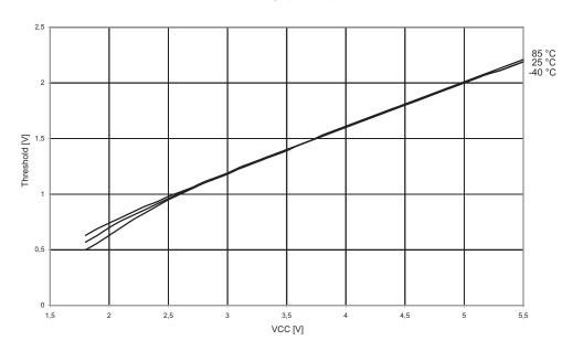
Figure 21-41. $V_{IH}$ - $V_{IL}$ : Input Hysteresis vs.  $V_{CC}$  (Reset Pin as I/O)
