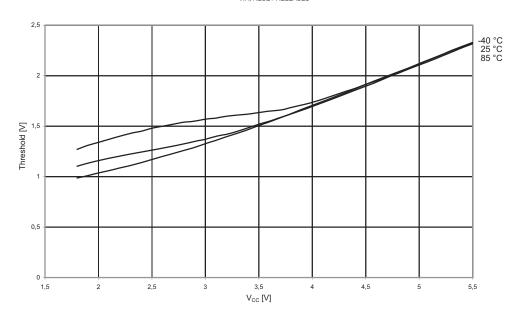
Figure 21-47.V $_{\rm IL}$ : Input Threshold Voltage vs. V $_{\rm CC}$  (Reset Pin, Read as '0')
