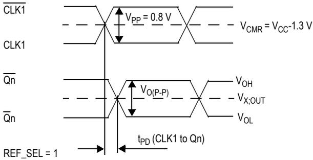
Figure 7. MC100ES8111 AC Reference Measurement Waveform (PECL Input)
