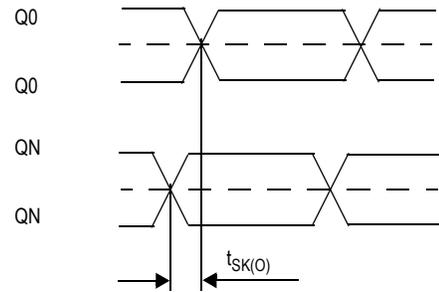
Figure 8. Output-to-Output Skew
