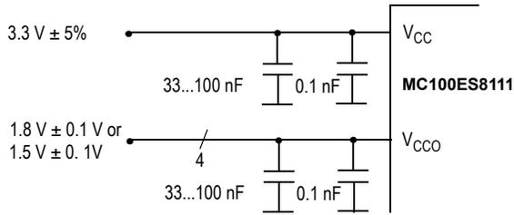
Figure 4.  $V_{CC}$ ,  $V_{CCO}$  Power Supply Bypass
