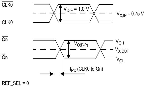
Figure 6. MC100ES8111 AC Reference Measurement Waveform (HSTL Input)
