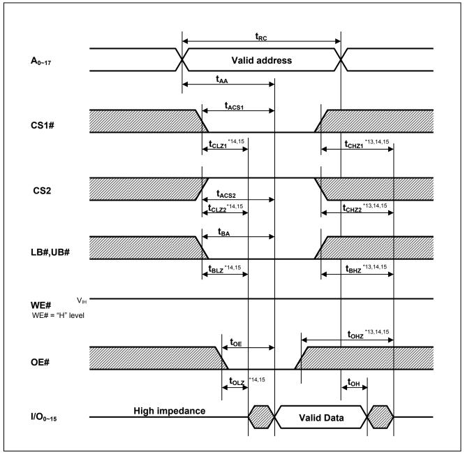
Note 13.  $t_{CHZ1}$ ,  $t_{CHZ2}$ ,  $t_{BHZ}$  and  $t_{OHZ}$  are defined as the time when the I/O pins enter a high-impedance state and are not referred to the I/O levels.
