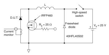
Fig. 8 - Unclamped Inductive Test Circuit
