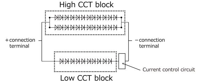
High CCT block 12 series  $\times$  2 parallel = 24 pcs of LEDs Low CCT block 10 series  $\times$  1 parallel = 10 pcs of LEDs
