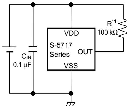
\*1. Resistor (R) is unnecessary for the CMOS output product.
