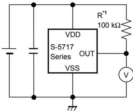
\*1. Resistor (R) is unnecessary for the CMOS output product.
