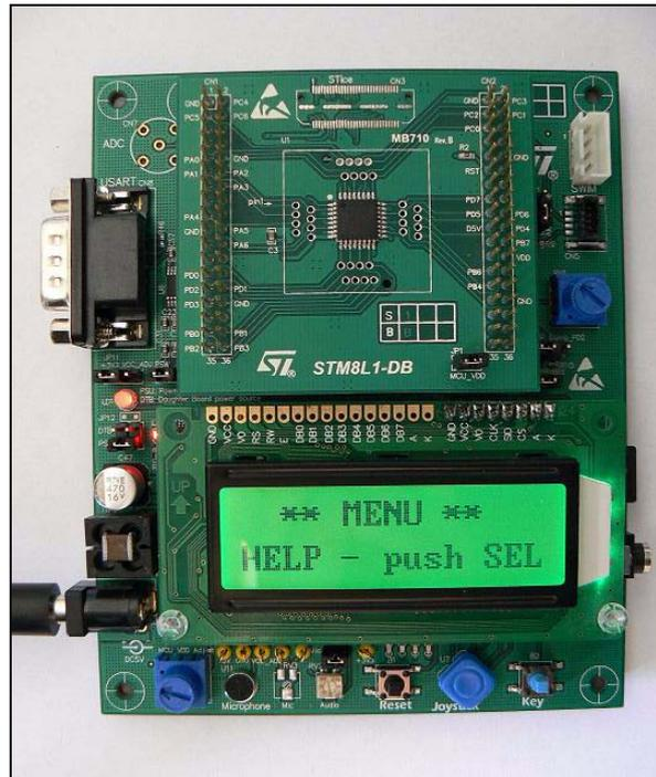
The full range of hardware features on the STM8L101-EVAL helps you to evaluate all peripherals (micro SD Card, USART, EEPROM, LCD, for example) and develop your own applications.
