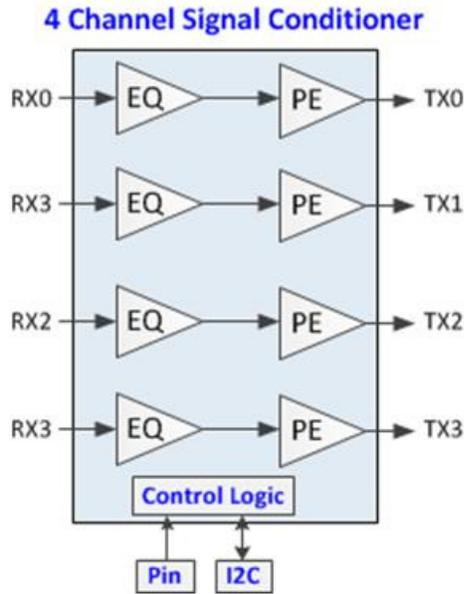
Figure 1: HMC7545AxLP47 4-Channel Signal Conditioner: Functional Diagram
