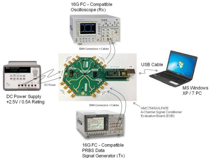
**Figure 6. HMC7545AxLP47 EVB Test Equipment Setup: Physical Diagram**
