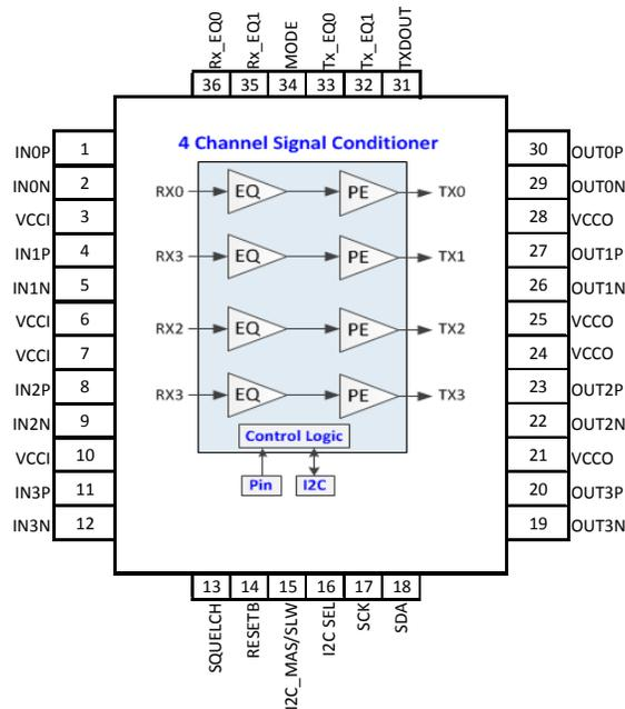
**Figure 2: HMC7545AxLP47 4-Channel Signal Conditioner: Pin Names**
