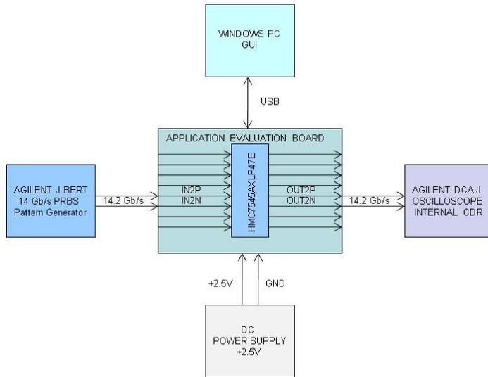
**Figure 5. HMC7545AxLP47 EVB Test Equipment Setup: Block Diagram**
