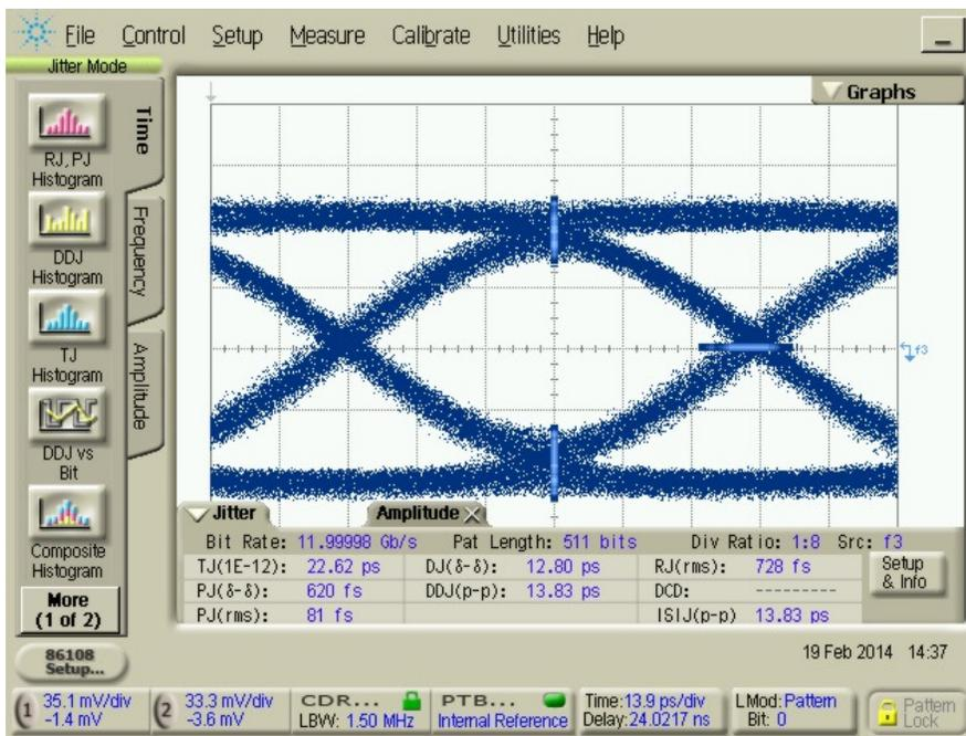
**Figure 19. 12.0 Gb/s PRBS 2<sup>9</sup>-1. HMC7545ABLP47 EVB with 10” Load Board Lossy Channel at Output Using 4-Channel Signal Conditioner De-Emphasis (DE), as Indicated by Point 4 in Figure 15.**
