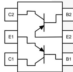
Figure 2. Internal Connections
