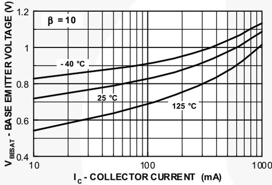
Figure 5. Base-Emitter Saturation Voltage vs. Collector Current
