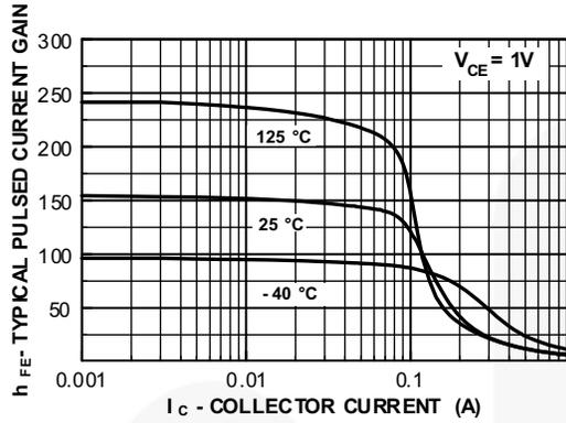
Figure 3. Typical Pulsed Current Gain vs. Collector Current
