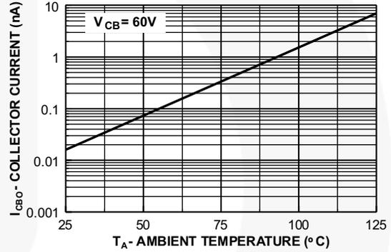
Figure 6. Collector Cut-Off Current vs. Ambient Temperature
