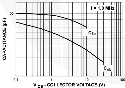
Figure 7. Input and Output Capacitance vs. Reverse Voltage
