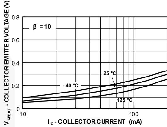
Figure 4. Collector-Emitter Saturation Voltage vs. Collector Current
