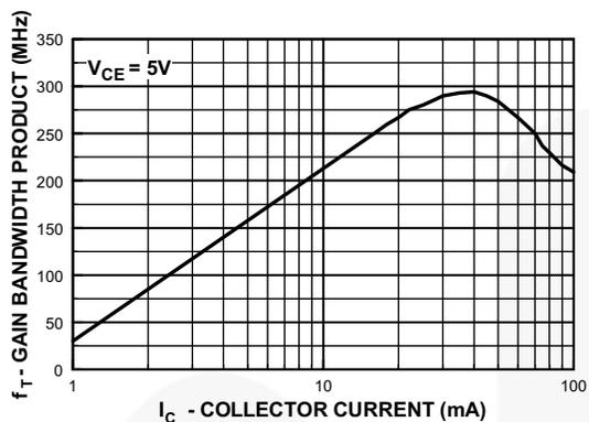
Figure 9. Gain Bandwidth Product vs. Collector Current
