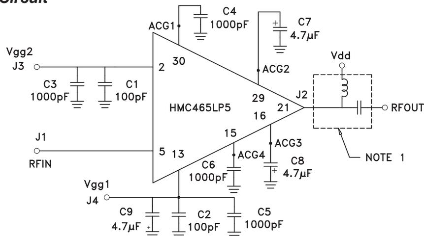
NOTE 1: Drain Bias (Vdd) must be applied through a broadband bias tee or external bias network.
