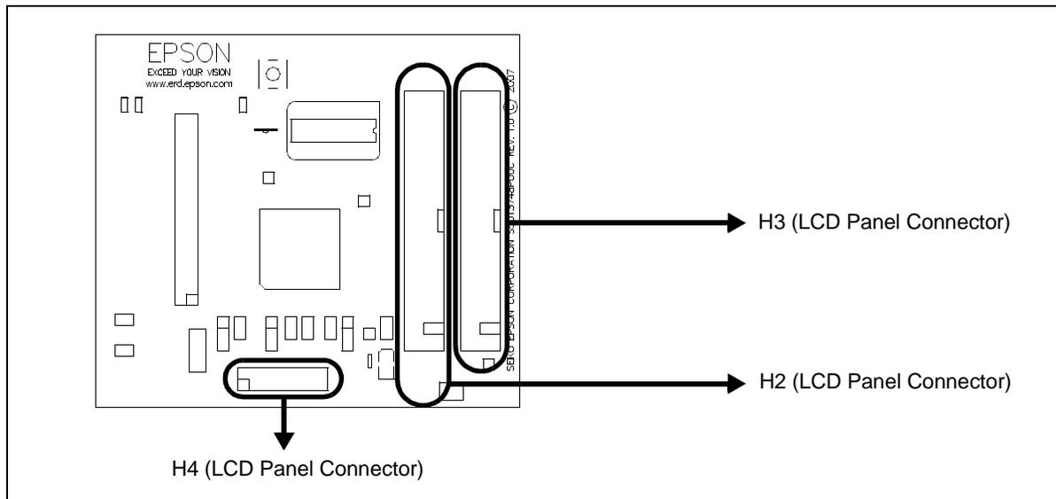
Figure 4-4: LCD Panel Connectors Location (H2, H3, H4)
