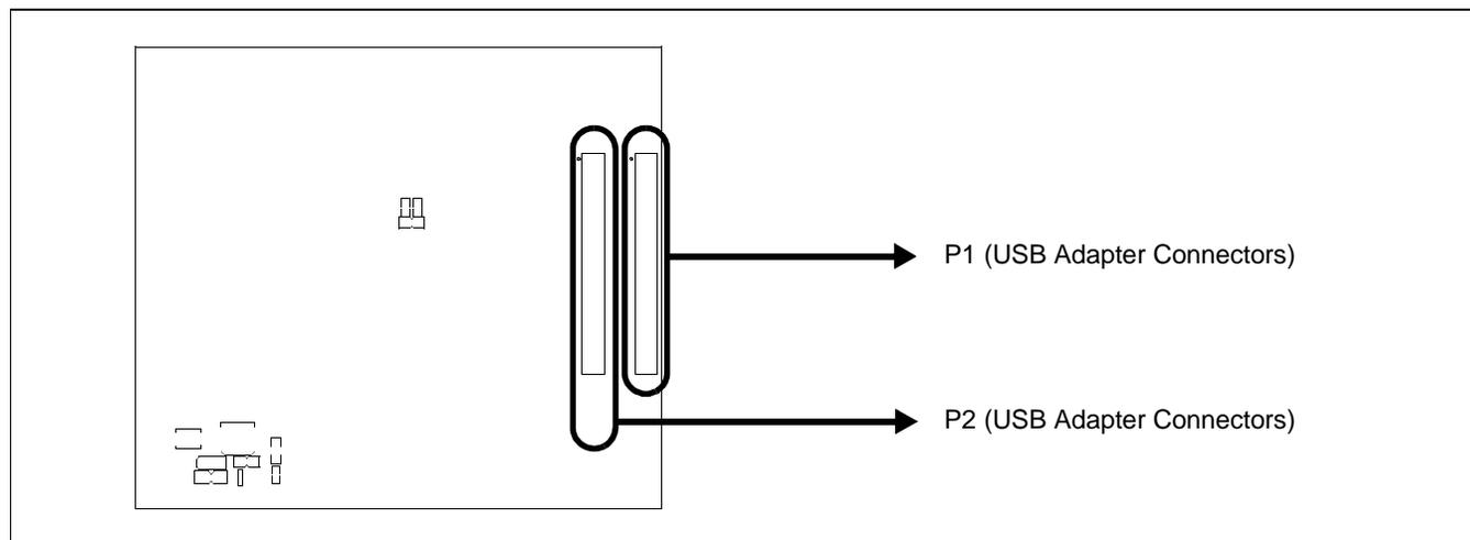
*Figure 4-3: USB Adapter Connector Locations (P1 and P2)*
