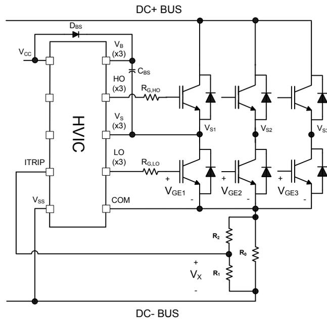
**Figure 19: Separate  $V_{SS}$  and  $V_{SO}$  (COM) pins**
