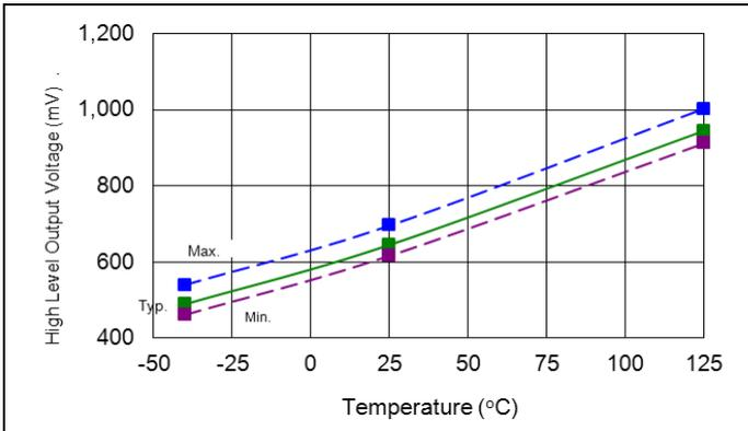
**Figure 48. High level output voltage vs. temperature**
