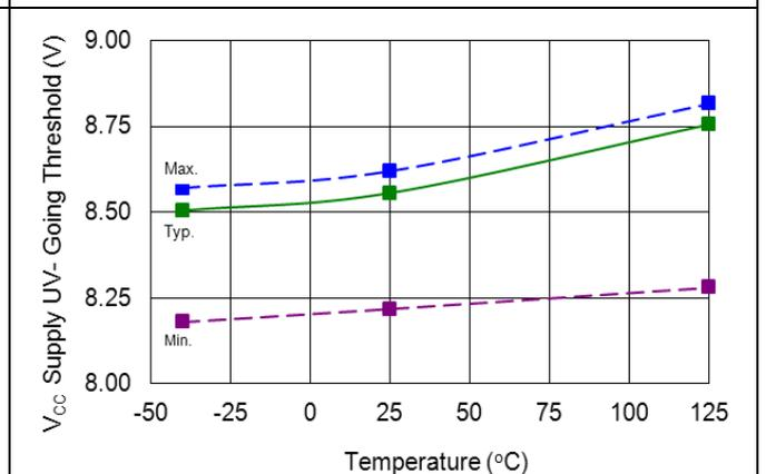
**Figure 51. V<sub>CC</sub> supply undervoltage negative going threshold vs. temperature**
