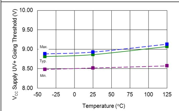
**Figure 50. V<sub>CC</sub> supply undervoltage positive going threshold vs. temperature**
