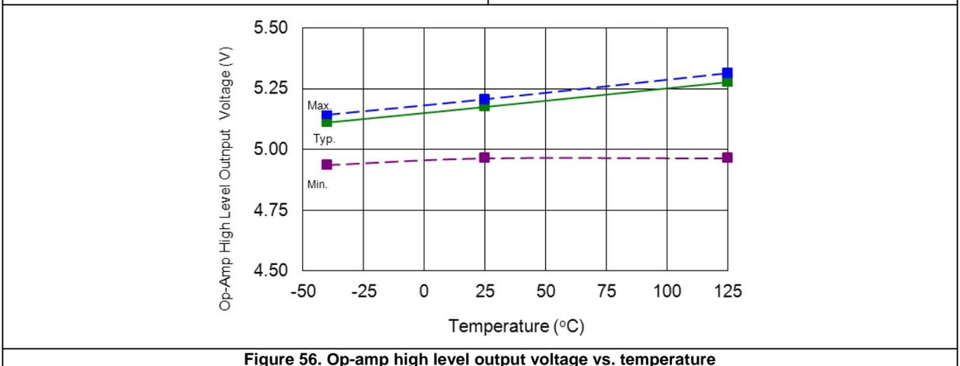
**Figure 56. Op-amp high level output voltage vs. temperature**
