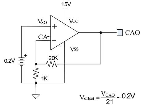
**Figure 31: Operational Amplifier Input Offset Voltage measurement**
