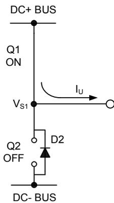
**Figure 21: Q1 conducting**
