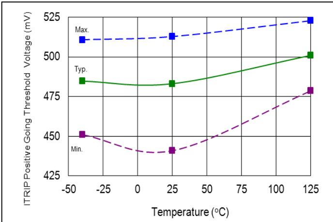
**Figure 54. ITRIP input positive going threshold vs. temperature**
