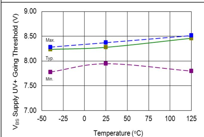
**Figure 52. V<sub>BS</sub> supply undervoltage positive going threshold vs. temperature**
