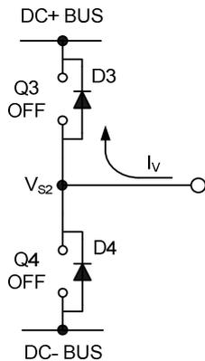
**Figure 23: D3 conducting**
