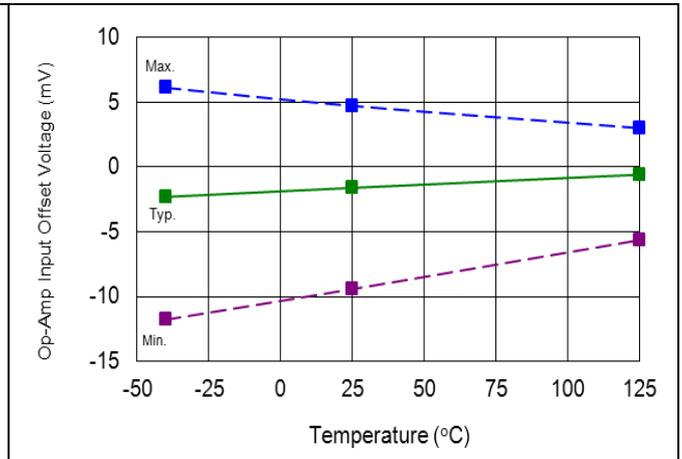
**Figure 55. Op-amp input offset voltage vs. temperature**
