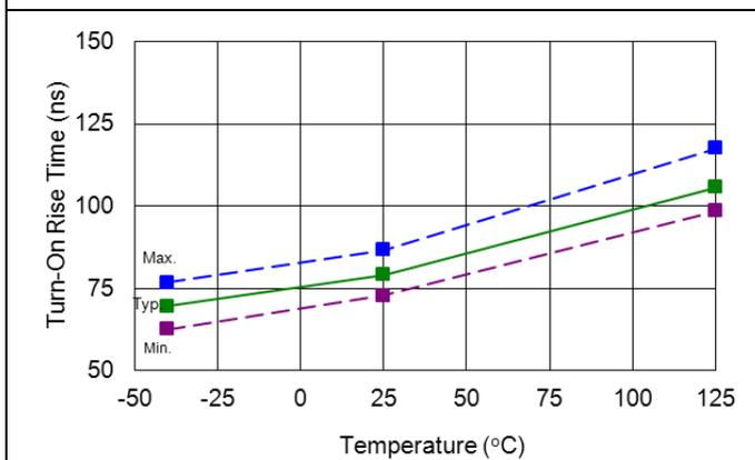
**Figure 40. Turn-on rise time vs. temperature**
