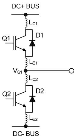
**Figure 25: Parasitic Elements**
