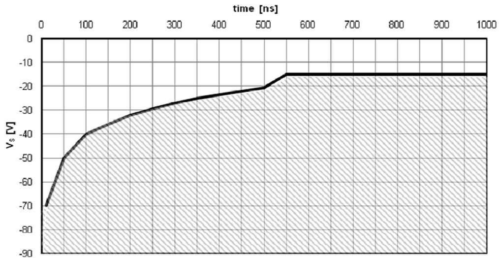
**Figure 28: Negative  $V_S$  transient SOA for AUIRS2332J**
