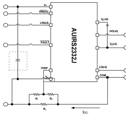
**Figure 35: Supply capacitor**
