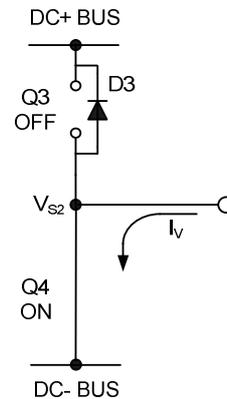
**Figure 24: Q4 conducting**
