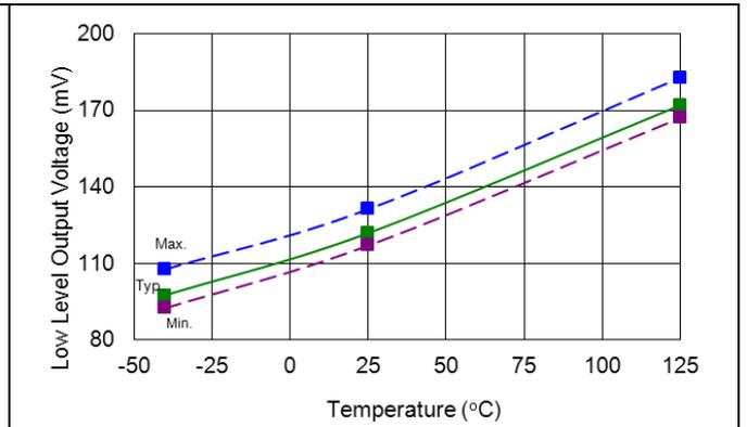
**Figure 49. Low level output voltage vs. temperature**
