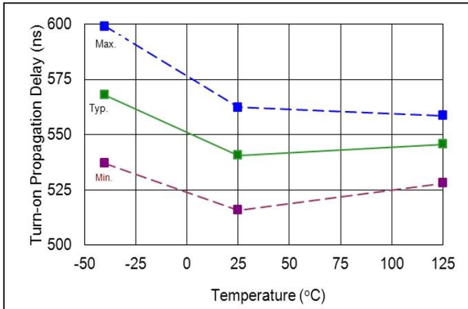
**Figure 38. Turn-on propagation delay vs. temperature**
