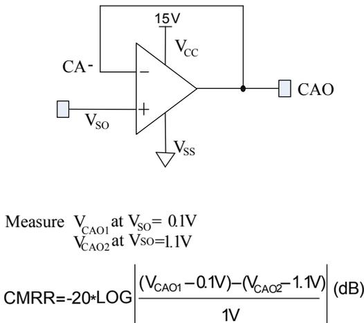
**Figure 32: Operational Amplifier Common mode rejection measurement**
