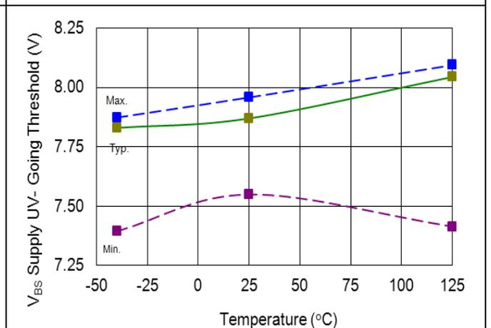
**Figure 53. V<sub>BS</sub> supply undervoltage negative going threshold vs. temperature**
