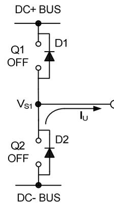
**Figure 22: D2 conducting**
