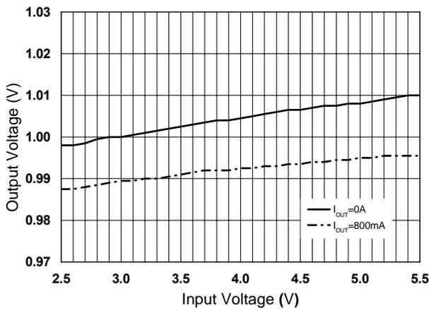
Figure 14. Line Regulation ( $V_{OUT}=1.0\pm 0.03V$ )
