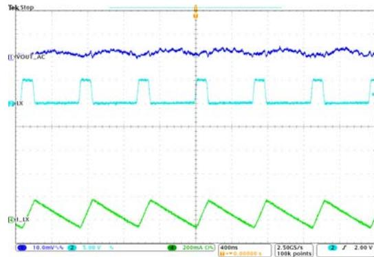
Figure 33. Output Ripple Voltage
