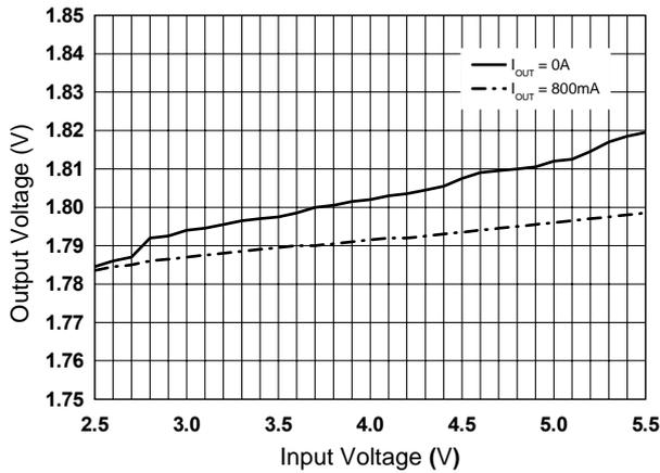
Figure 16. Line Regulation ( $V_{OUT}=1.8\pm 0.03V$ )
