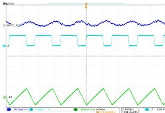
Figure 34. Output Ripple Voltage
