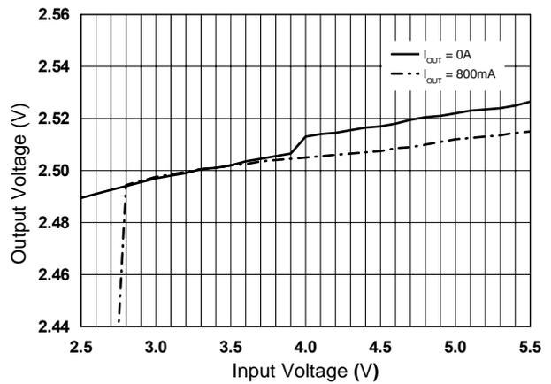
Figure 17. Line Regulation ( $V_{OUT}=2.5\pm 0.03V$ )
