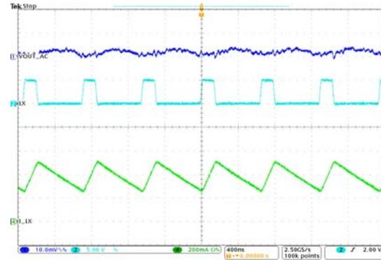
Figure 35. Output Ripple Voltage
