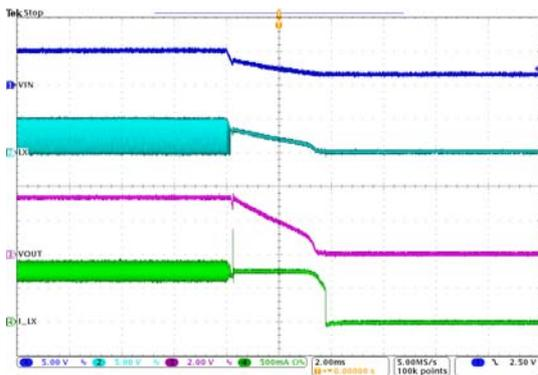
Figure 26. Shut Down through VIN
