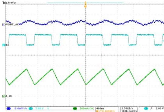
Figure 36. Output Ripple Voltage
