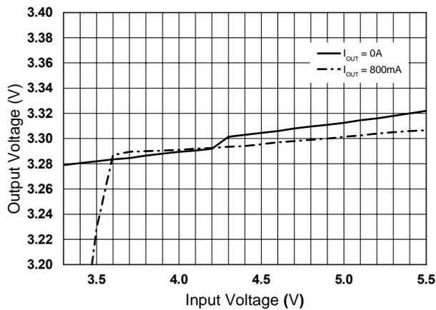
Figure 18. Line Regulation ( $V_{OUT}=3.3\pm 0.03V$ )
