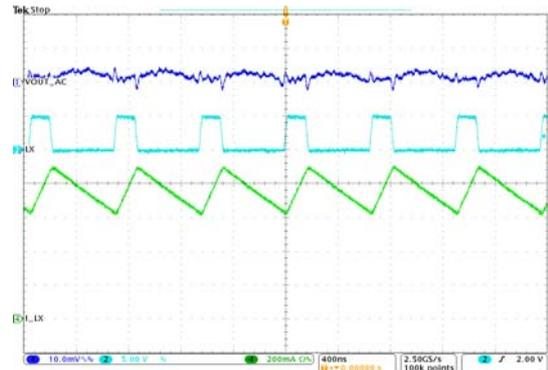
Figure 37. Output Ripple Voltage
