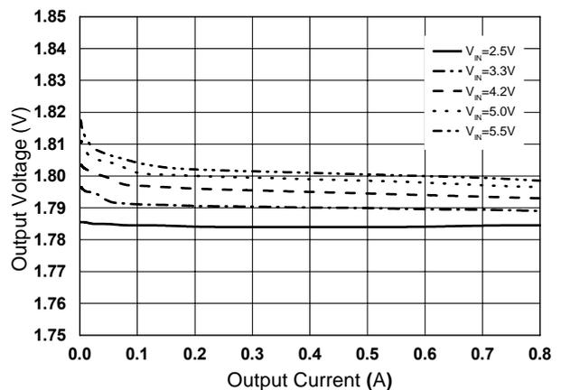
Figure 11. Load Regulation ( $V_{OUT}=1.8\pm 0.03V$ )
