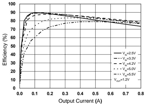
Figure 5. Efficiency vs. Output Current ( $V_{OUT}=1.2V$ )
