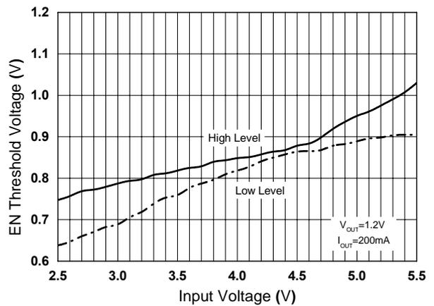
Figure 19. EN Threshold Voltage vs. Input Voltage
