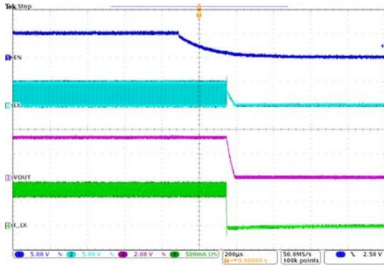
Figure 24. Shut Down through EN
