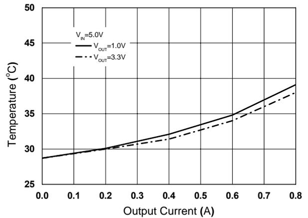
Figure 21. Temperature vs. Output Current
