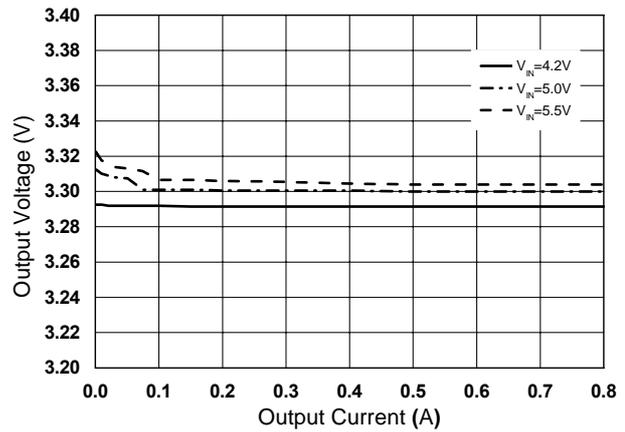
Figure 13. Load Regulation ( $V_{OUT}=3.3\pm 0.03V$ )
