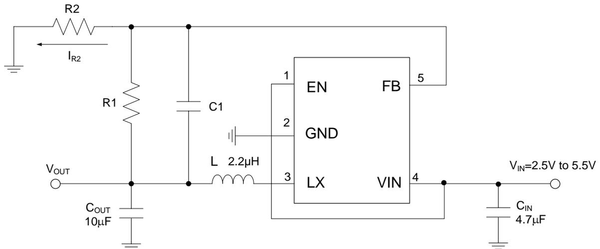
Note 2:  $V_{OUT1} = V_{REF} \times \left(1 + \frac{R_1}{R_2}\right)$ .
