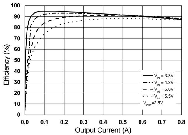
Figure 7. Efficiency vs. Output Current ( $V_{OUT}=2.5V$ )
