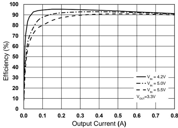
Figure 8. Efficiency vs. Output Current ( $V_{OUT}=3.3V$ )
