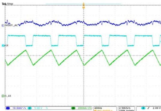
Figure 38. Output Ripple Voltage
