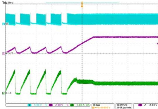
Figure 28. Short Circuit Recovery
