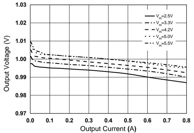
Figure 9. Load Regulation ( $V_{OUT}=1.0\pm 0.03V$ )
