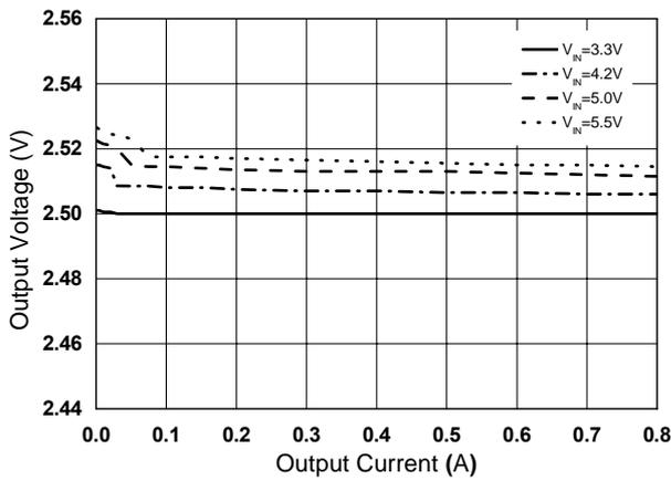
Figure 12. Load Regulation ( $V_{OUT}=2.5\pm 0.03V$ )
