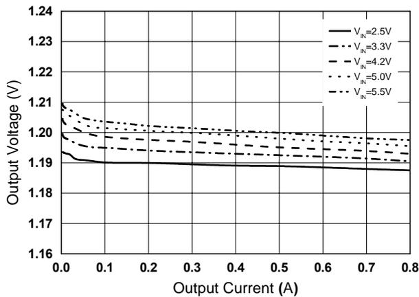
Figure 10. Load Regulation ( $V_{OUT}=1.2\pm 0.03V$ )
