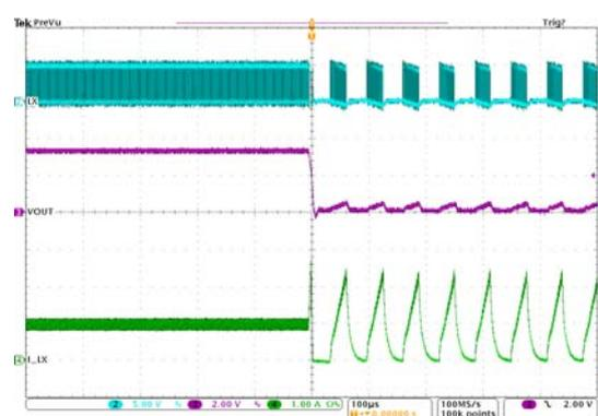
Figure 27. Short Circuit Protection
