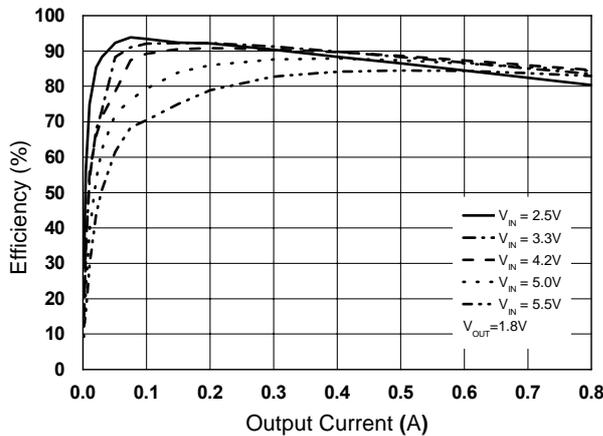
Figure 6. Efficiency vs. Output Current ( $V_{OUT}=1.8V$ )
