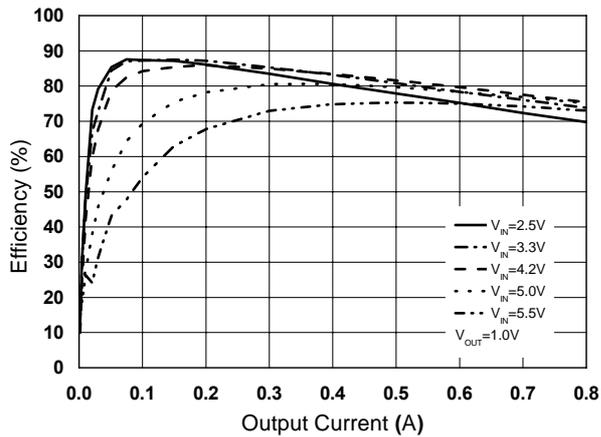
Figure 4. Efficiency vs. Output Current ( $V_{OUT}=1.0V$ )
