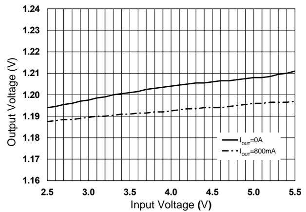
Figure 15. Line Regulation ( $V_{OUT}=1.2\pm 0.03V$ )
