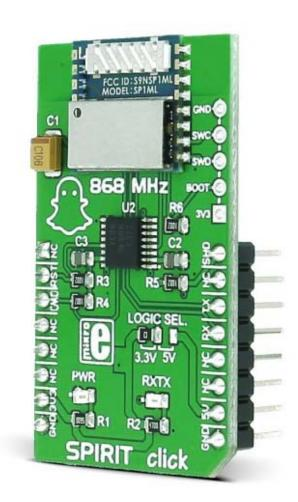
**SPIRIT click** carries the SP1ML 868MHz ultra low-power RF module. The board is designed to use 3.3V power supply and 3.3V or 5V I/O voltage levels. It communicates with the target MCU over UART interface, with additional functionality provided by the following pins on the mikroBUS<sup>TM</sup> line: PWM, RST, CS.
