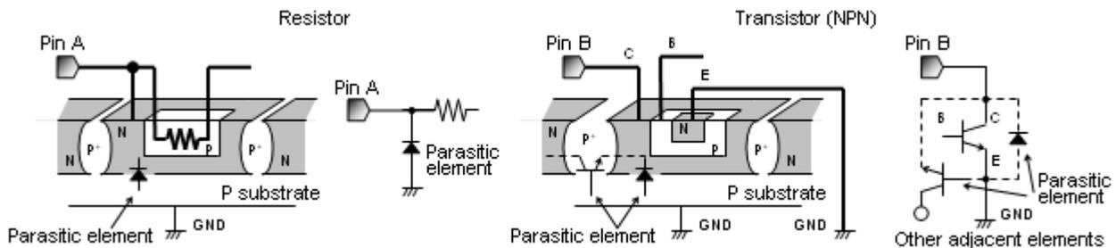
Fig.36 Simplified structure of monolithic IC
