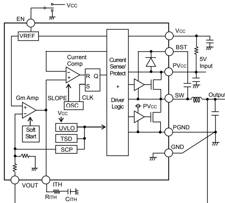
Fig.3 Block Diagram
