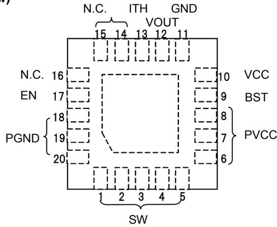
Fig.2 Pin configuration
