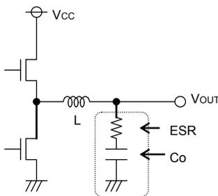
Fig.29 Output capacitor
