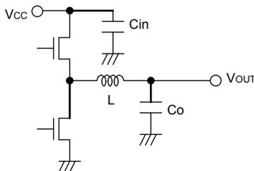
Fig.30 Input capacitor
