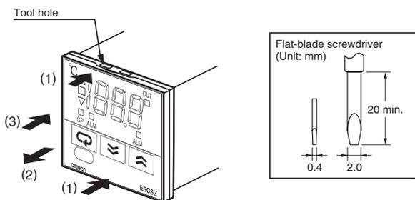
2. Insert the tool in the gap between the front panel and rear case, and pull out the front panel slightly. Grip the front panel and pull out fully. Be sure not to impose excessive force on the panel.
