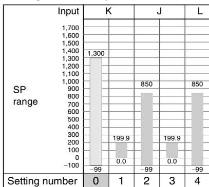
The shaded value indicates the default setting status. Do not set the temperature range switch to between No. 5 and No. 9.
