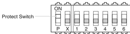
When the protect switch is ON, Up Key and Down Key operations are prohibited to prevent setting mistakes.
