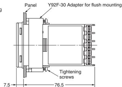
Note: 1. The recommended panel thickness is 1 to 4 mm.
