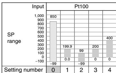
The shaded value indicates the default setting status. Do not set the temperature range switch to between No. 5 and No. 9.
