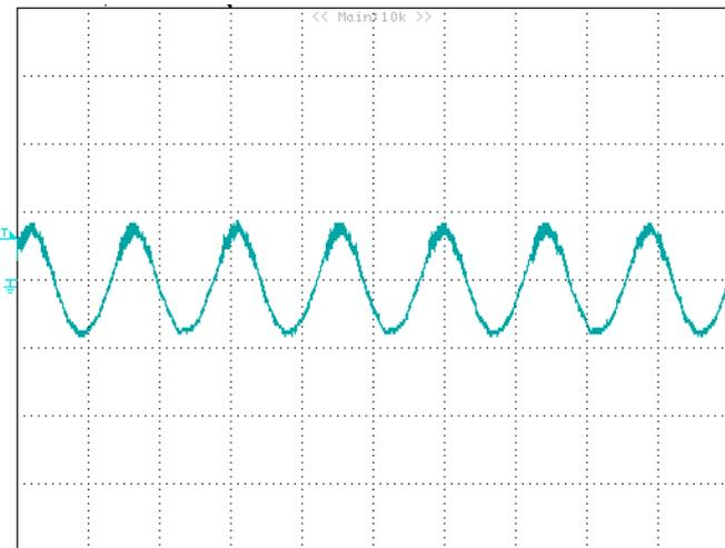
**Figure 14:** Output voltage ripple at nominal input voltage and rated load current ( $I_o=20\text{A}$ ) ( $50\text{mV}/\text{div}$ ,  $2\mu\text{s}/\text{div}$ )
