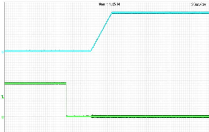
**Figure 4:** Turn-on transient at zero load current (20ms/div).
