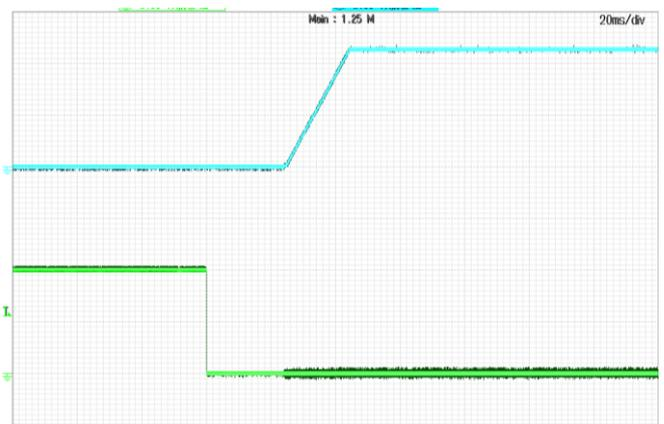
**Figure 5:** Turn-on transient at full rated load current (20ms/div).
