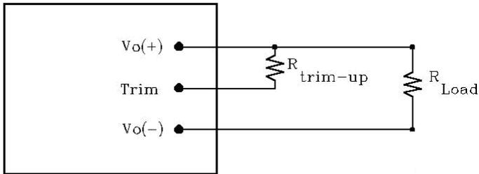
**Figure 19:** Circuit configuration for trim-up (increase output voltage)
