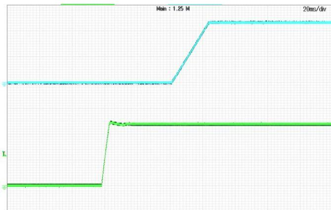
**Figure 6:** Turn-on transient at zero load current (20 ms/div).
