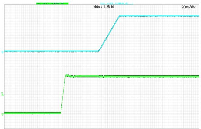
**Figure 7:** Turn-on transient at full rated load current (20 ms/div).
