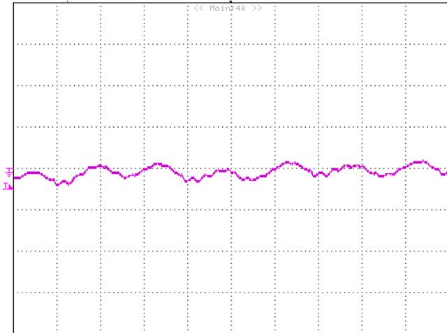
**Figure 12:** Input reflected ripple current,  $i_s$ , through a  $12\mu\text{H}$  source inductor at nominal input voltage and rated load current ( $20\text{mA}/\text{div}$ ,  $2\mu\text{s}/\text{div}$ ).
