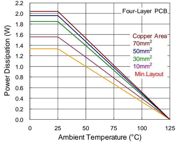
Figure 7. Derating Curves for RT8295B Package
