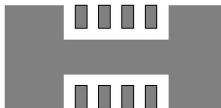
(e) Copper Area = 70mm<sup>2</sup>,  $\theta_{JA} = 49^{\circ}\text{C/W}$
