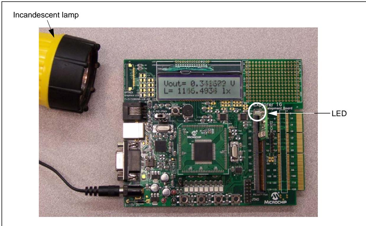
**FIGURE 2-2:** MCP6031 Photodiode PICtail™ Plus Demo Board Operation.
