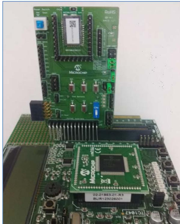
Figure 29: Explorer 16 Development Board with RN4870 PICtail Plus
