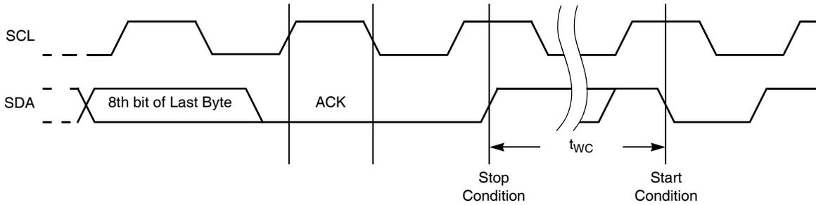
Nonvolatile Write Cycle Timing
