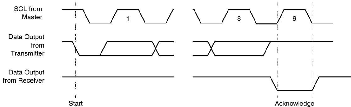
Figure 8. Byte Write Sequence
