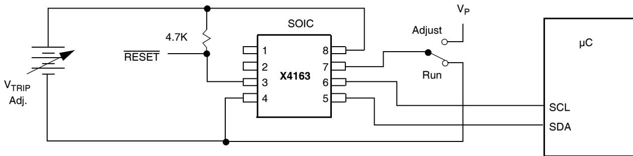
Figure 4.  $V_{TRIP}$  Programming Sequence
