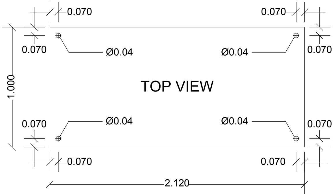
Figure 2.2 EVB-LAN9500A-LC Mechanicals
