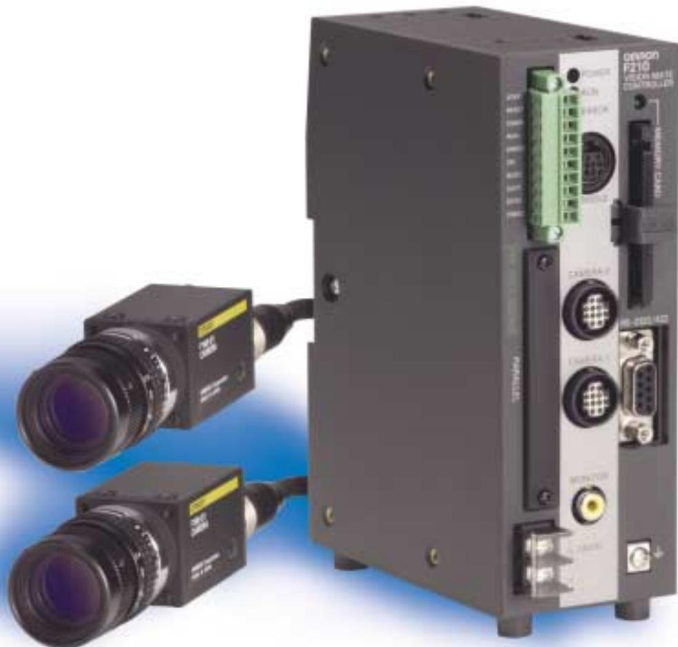
*Advanced machine vision capability for high-speed, two-camera applications in a compact package*
