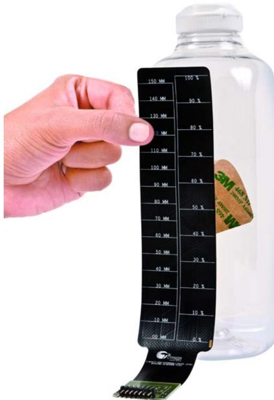
2. Thoroughly press the entire sensor area to the container to ensure there are no air bubbles in the adhesive layer. Air bubbles allow the distance between the sensor and the liquid to fluctuate. Distance changes cause changes to the sensor's capacitance resulting in reduced liquid level accuracy. Air bubbles can be observed through the adhesive layer on the back of the sensor through the bottle.
