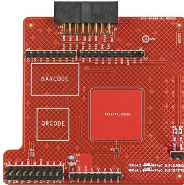
Figure 2-3. Top View of both CY8CKIT-022 Sensors
