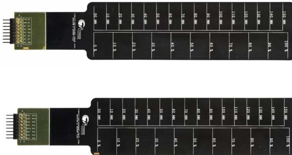
Figure 2-4. Bottom View of both CY8CKIT-022 Sensors
