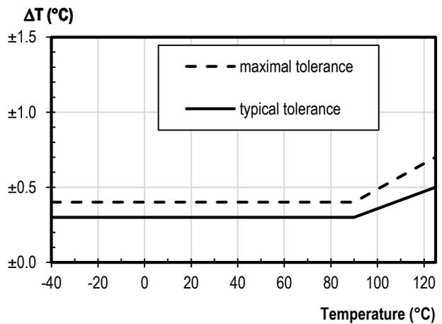
**Figure 7** Temperature accuracy of the SHT31 sensor.
