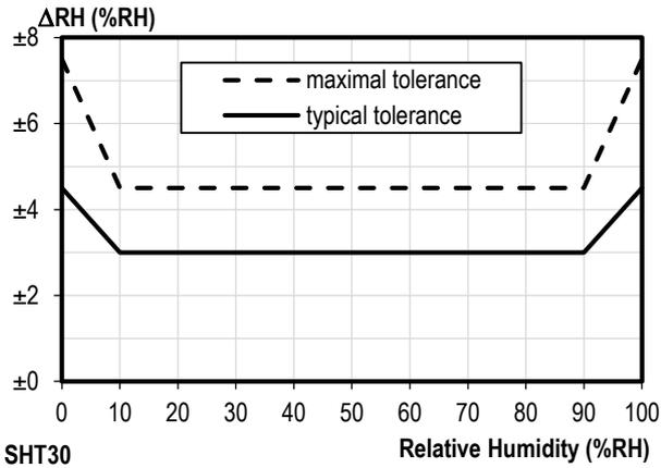
**Figure 2** Tolerance of RH at 25°C for SHT30
