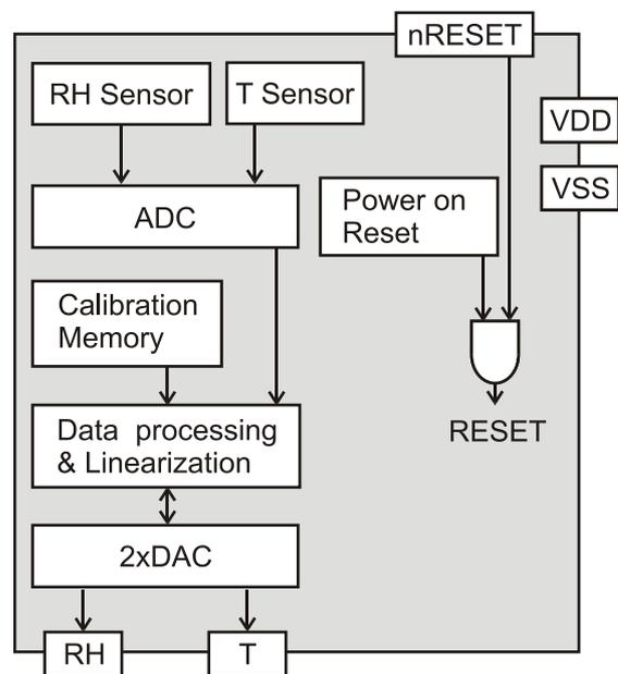
**Figure 1** Functional block diagram of the SHT3x-ARP. The sensor signals for humidity and temperature are factory calibrated, linearized and compensated for temperature and supply voltage dependencies.
