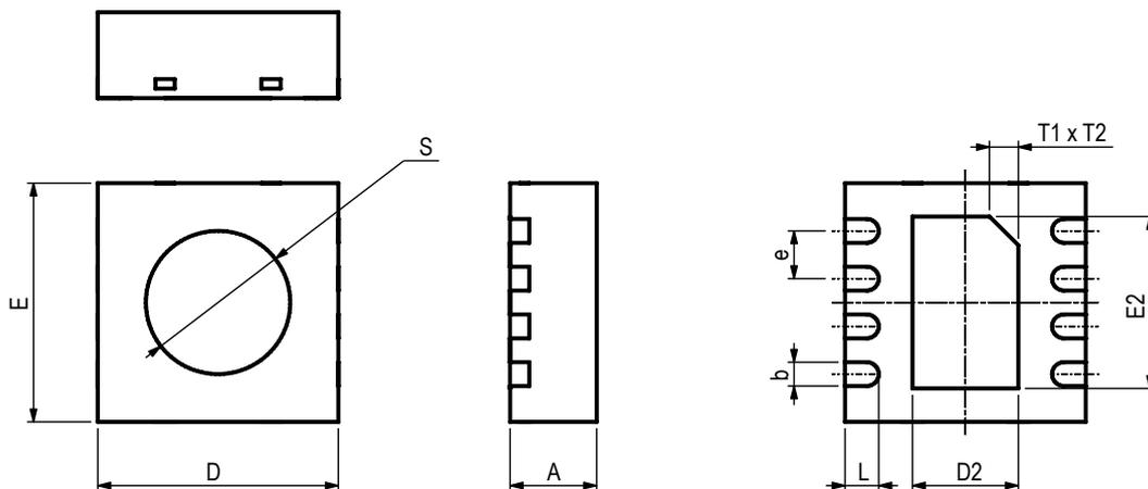
Figure 12 Dimensional drawing of SHT3x-ARP sensor package.
