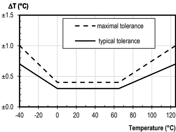
**Figure 6** Temperature accuracy of the SHT30 sensor.
