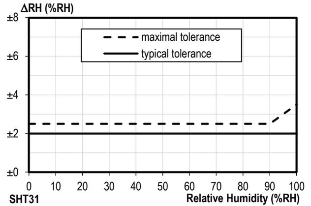
**Figure 3** Tolerance of RH at 25°C for SHT31
