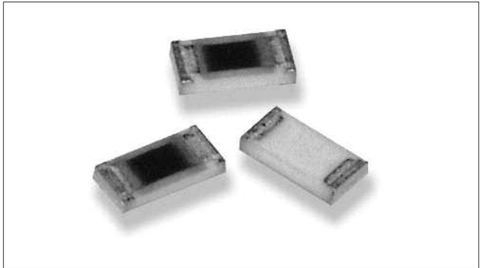
Precious metal terminations are screen printed onto a ceramic base and fired. The resistive element is screen printed and fired and the passivation layer added. Each resistor is trimmed to tolerance by sand blasting. The prescribed tile is broken into strips, the end plating is fired on and the strips broken into individual components. Final termination is made by electroplating.
