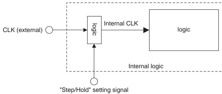
When the Step/Hold data is set to the Hold state, the state of the external clock signal (CLK) at that time is latched and held as the internal clock signal.
