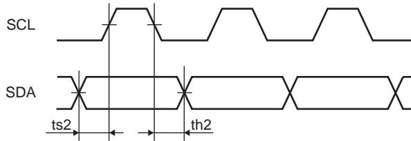
When data is not being transferred, both SCL and SDA are in the high state. The start condition is generated and access is started when SDA is changed from high to low while SCL and SDA are high. Conversely, the stop condition is generated and access is ended when SDA is changed from low to high while SCL is high.
