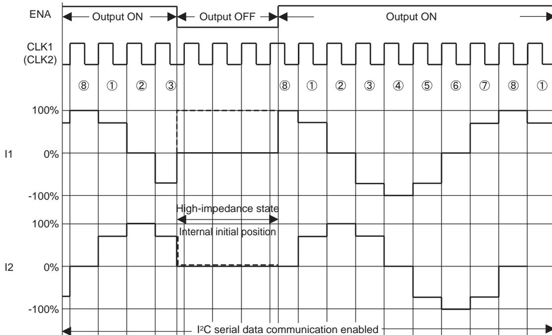
\* The output does not operate unless “output enable” is set to the “output ON” state using an I<sup>2</sup>C serial data communication.
