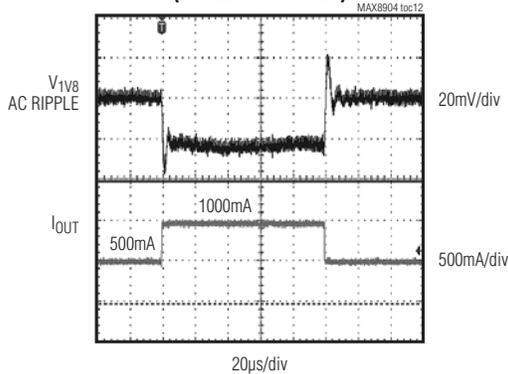
OUTPUT VOLTAGE LOAD REGULATION (1V8)
