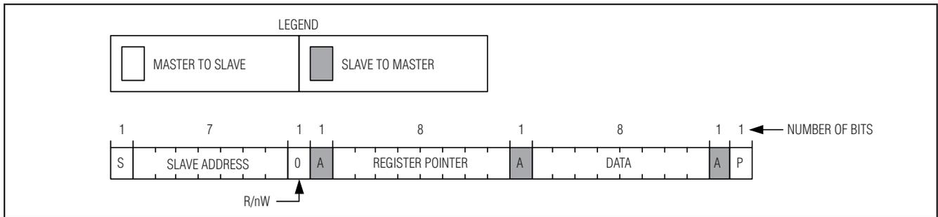
Figure 4. Write-Byte Format
