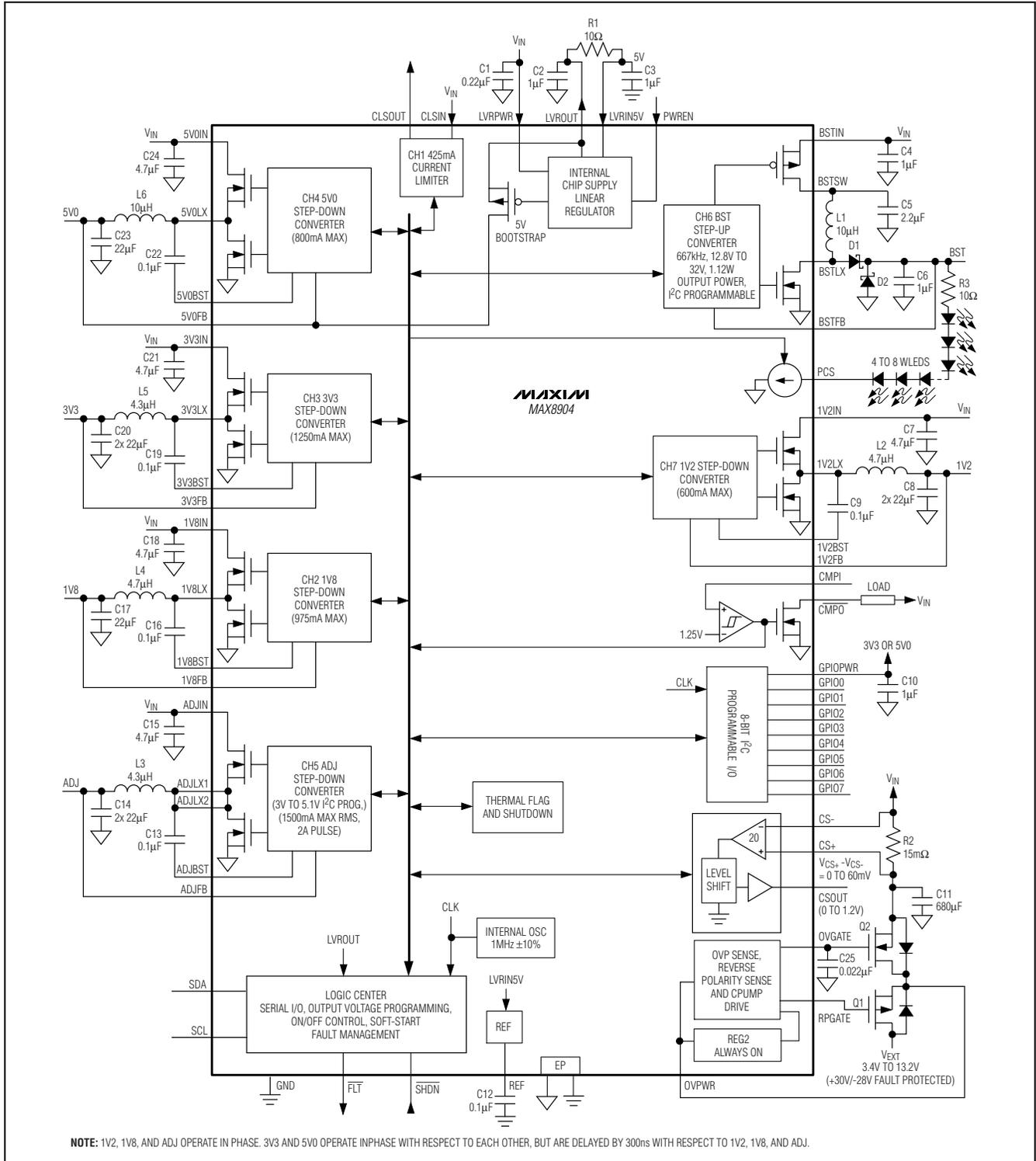
Figure 1. Typical Application Circuit and Function Diagram
