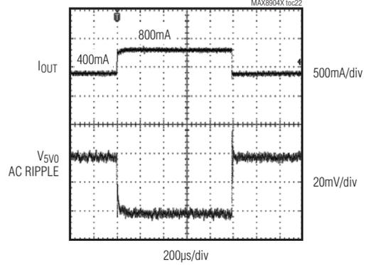
**OUTPUT VOLTAGE LOAD REGULATION (5V0)**
