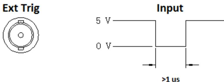
Figure 4-3 Trigger model
