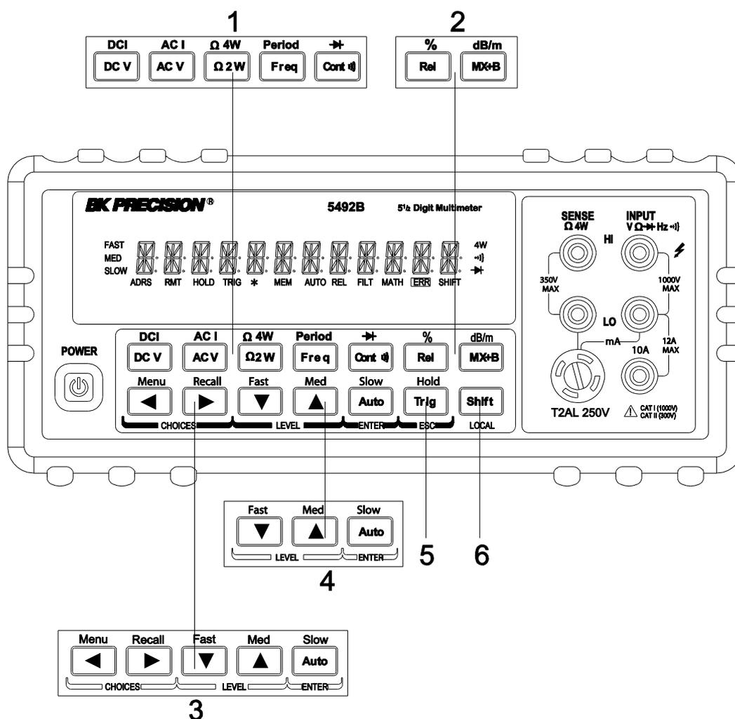
Figure 1 - Front Panel View
