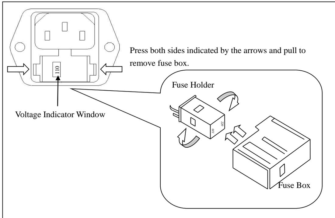
There is a second fuse with a fuse holder located in the front panel of the multimeter. This is an over current protection fuse for the low current measurement input. It is rated for a T2AL, 250 V fuse. To remove and replace this fuse, see the illustration below:
