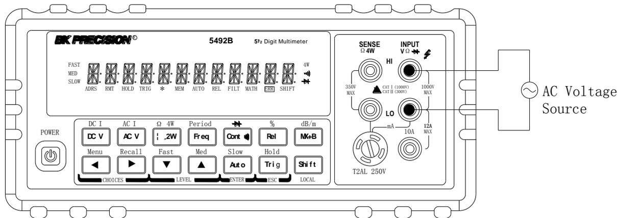
Input Impedance = 1 M $\Omega$  in parallel with <100 pF
