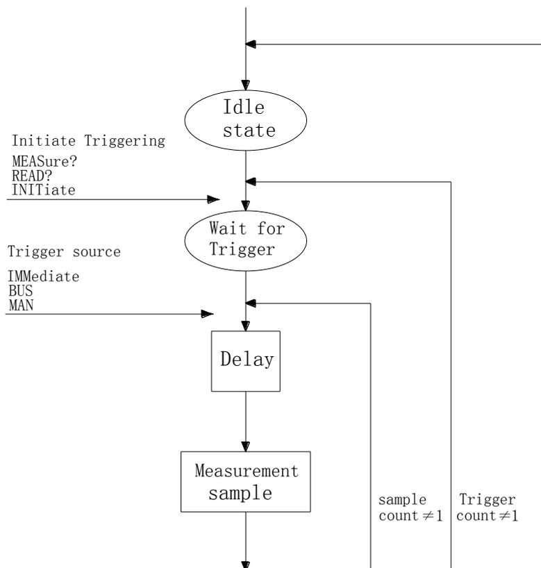
Figure 4-2 Trigger model
