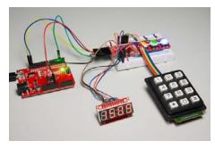
An SX1509 controlling three LEDs, monitoring three buttons and a 12-button keypad, and producing SPI signals to drive a Serial 7-Segment Display.
