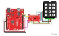
There isn't a lot of flexibility in the SX1509's keypad engine. The rows of you matrix have to be connected, sequentially, to pins 0-7, and the columns wire up to pins 8-15. Our four row buses must route to pins 0-3, and the three columns are connected to 8-10. That still leaves plenty of pins for LED driving!
