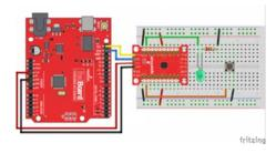
Match up 3.3V, GND, SDA, and SCL between your Arduino and the SX1509 Breakout. Then connect an LED to I/O 15 – you can either configure it to source or sink current. And connect an active-low button to I/O 0.
