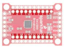
The SX1509 breaks its 16 I/O into two **banks** – bank A and bank B. Each bank can operate on a separate power supply, but by default they're both set to 3.3V. Bank A is powered by VCC1, and bank B is supplied by VCC2. VCC1 and VCC2 can range between 1.2V and 3.6V, if you want to supply them externally. Check out the "Jumpers" section for more information on that.
