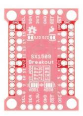
By default, these rails are both set to **ground** – handy if you want to fan out some active-low buttons, or current-sourced LEDs. Jumpers on the back side allow you to switch the rails from GND to either VCC1 or VCC2. You'll need to cut the jumper between GND and the rail, then blob solder between the rail and VCC.
