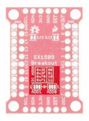
The board defaults each of those pins to GND, which sets the I<sup>2</sup>C address to **0x3E**. To set either jumper to "1" (HIGH), grab a hobby knife, cut the trace connecting to "0", and blob some solder between the center pad and "1".
