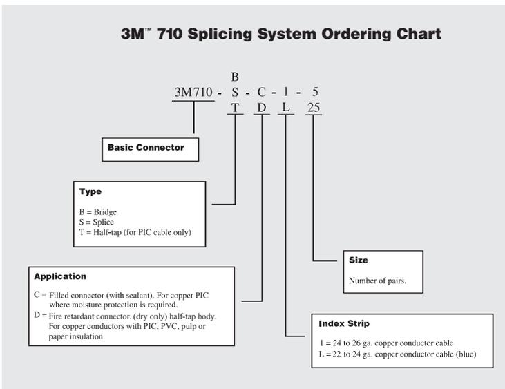
26/22 gauge (0.65 - 0.40 mm) connectors are standard. \*3M™ Scotchlok™ Connectors UY2 recommended for 19 AWG (0.9 mm) solid polypropylene insulated conductors.
