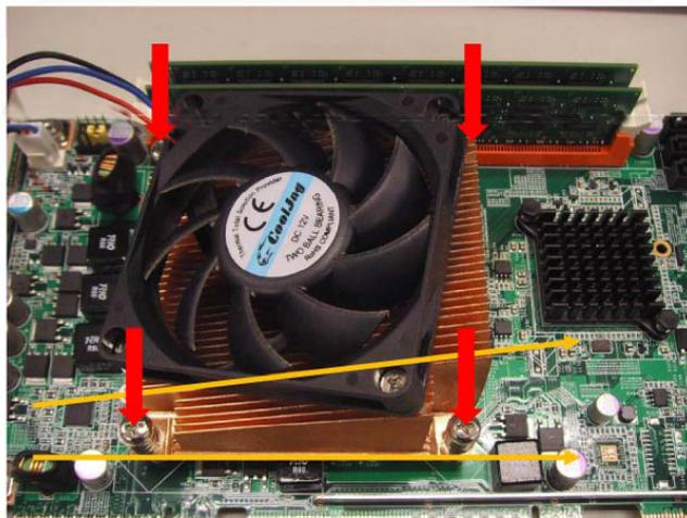
Note the direction of CPU cooler; it must follow the diagram shown above. Installing a CPU cooler in the wrong direction may cause poor heat dissipation that could damage the CPU card.
