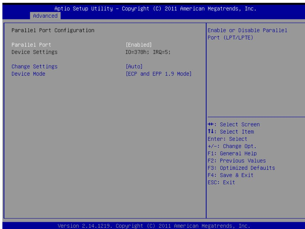
**Figure 3.18 Parallel Configuration**
