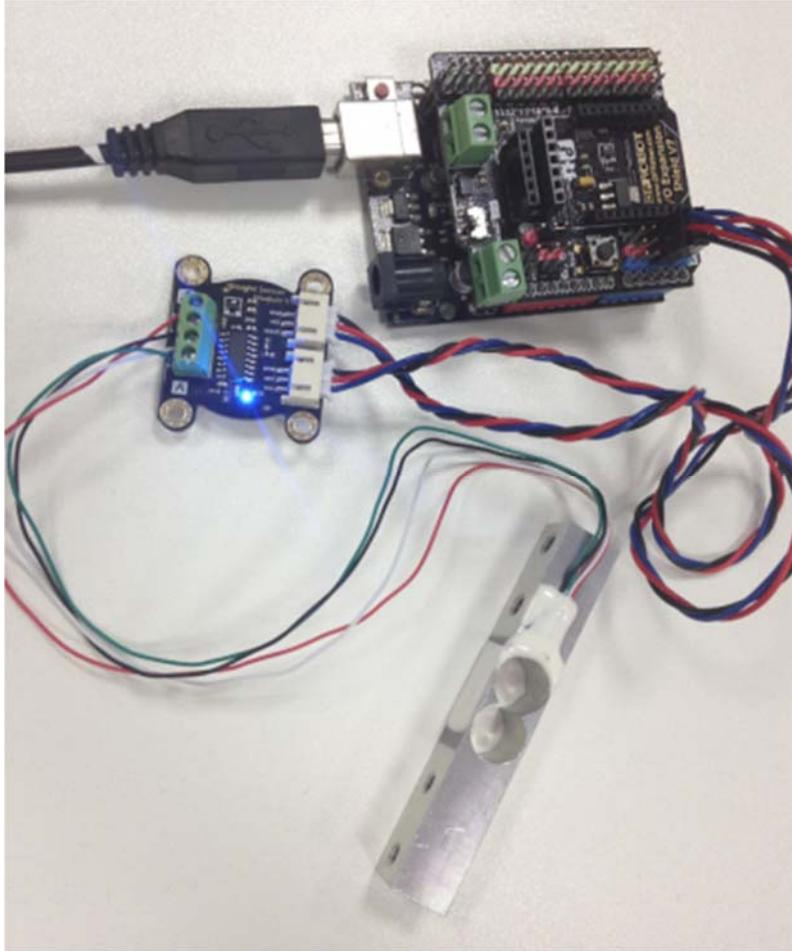
Physical wiring diagram
