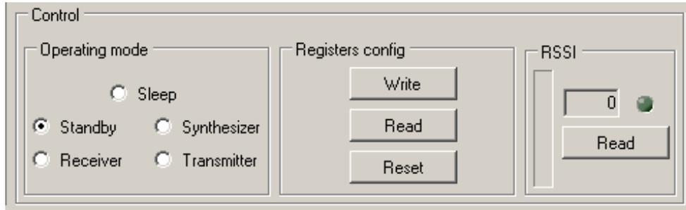
**Figure 30. The Mode Control Box also Incorporates RSSI**
