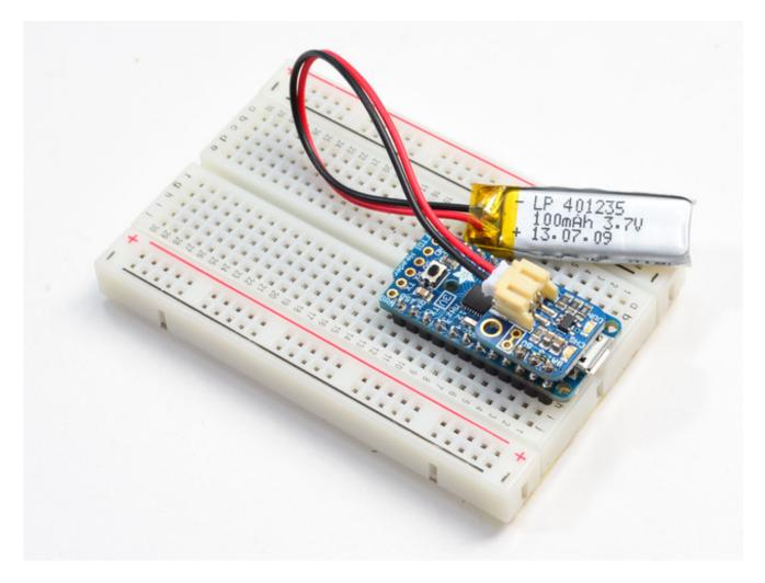
If you have a Pro Trinket you probably know it's the perfect little size for a portable project. This LiPoly backpack makes it really easy to do! Instead of wiring 2 or 3 boards together to make a charging system, this little PCB sits on top of the Pro Trinket and allows a LiPoly/Lilon battery to plug in. When the Pro Trinket USB port is powered, the battery is recharged automatically. Unplug the USB port and the Pro Trinket will switch over to the rechargeable battery.
