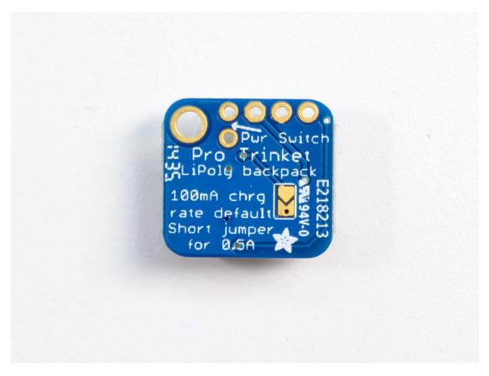
For use with Adafruit LiPoly/Lilon batteries only! Other batteries may have different voltage, chemistry, polarity or pinout.
