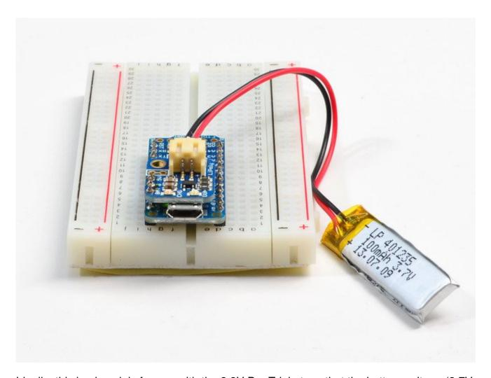
Ideally, this backpack is for use with the 3.3V Pro Trinket, so that the battery voltage (3.7V-4.2V) will get regulated down to 3.3V on the Pro Trinket board. However, many times, you can run a 5V Pro Trinket + accessories off of the ~4V from the LiPoly battery with no problem. (Technically its overclocking but we've never seen that affect the Pro Trinket itself, AVRs are happy to overclock without complaint).
