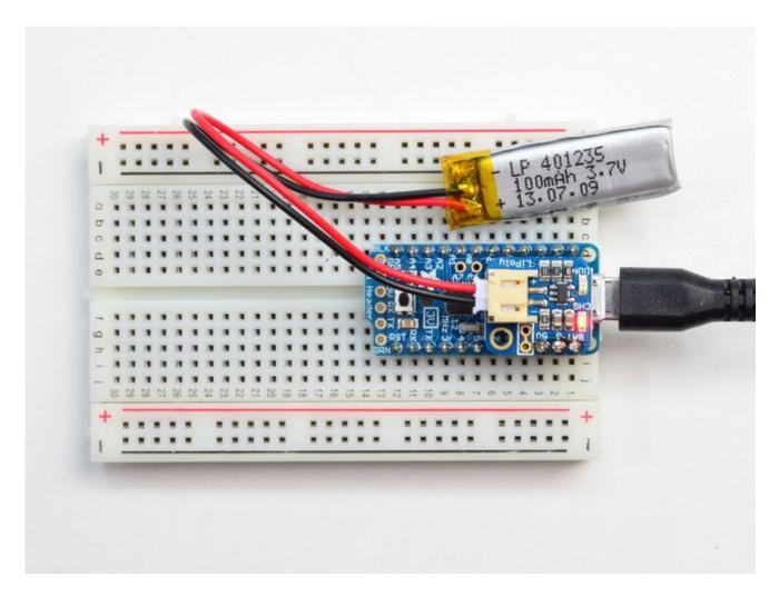
If you want to add an On/Off switch, we also made that really easy. The two 0.1" holes with a box around them are the battery output line. Carefully cut the trace between them with a hobby knife and replace with two wires from a switch like this slide switch (http://adafru.it/drN), or this pushbutton one (http://adafru.it/1683), for example.
