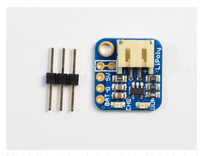
Solder the backpack on with the extra long header so that it can still plug into a breadboard, or clip the long header leads short afterwards for a slim package. There are two LEDs - one red and one green. While charging, the red LED is lit. When the battery is fully charged and ready for use, the green LED turns on. Seriously, it could not get more easy.
