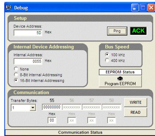
Figure 29. Evaluation Software I<sup>2</sup>C Debug Window
