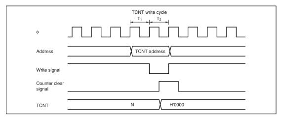
Figure 10.45 Contention between TCNT Write and Clear Operations
