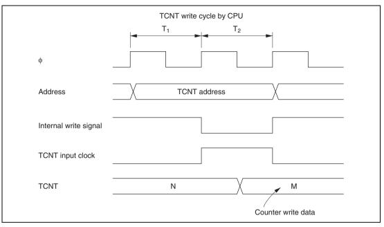
Figure 11.11 Contention between TCNT Write and Increment
