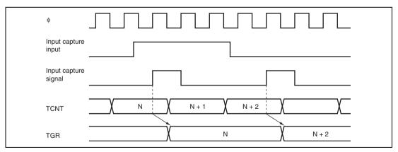
Figure 10.33 Input Capture Input Signal Timing
