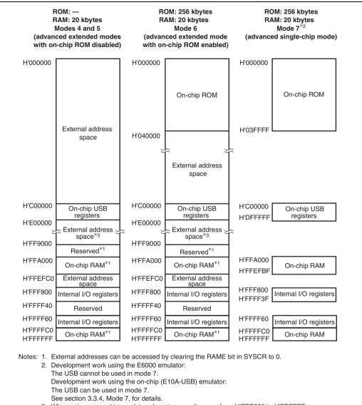
3. When using an on-chip emulator, do not access the area from H'FEE800 to H'FEFFFF.
