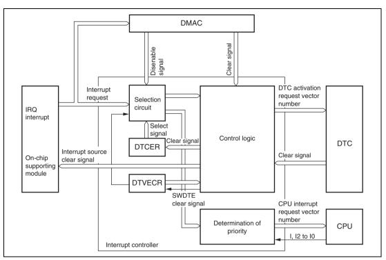
Figure 5.7 Interrupt Control for DTC and DMAC
