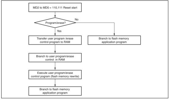
Figure 19.8 Programming/Erasing Flowchart Example in User Program Mode
