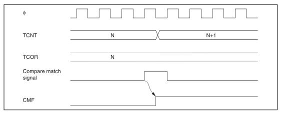
Figure 11.5 Timing of CMF Setting
