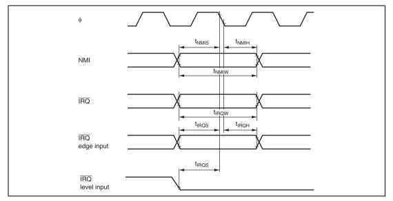
Figure 25.6 Interrupt Input Timing
