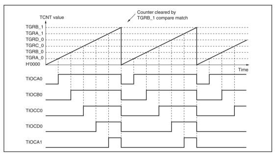
Figure 10.23 Example of PWM Mode Operation (2)
