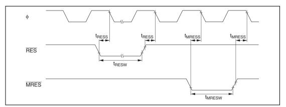
Figure 26.5 Reset Input Timing
