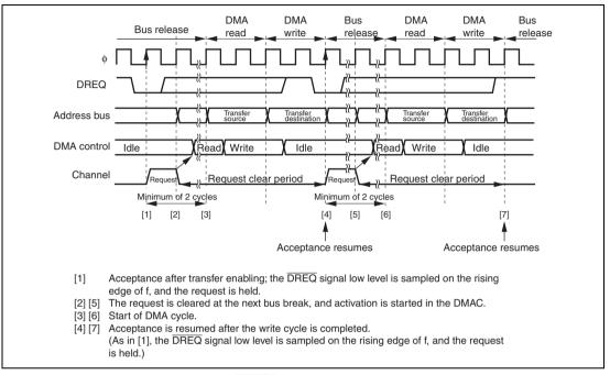
Figure 7.20 shows an example of  $\overline{\text{DREQ}}$  level activated normal mode transfer.
