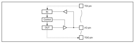
Figure 14.2 Boundary Scan Register Configuration
