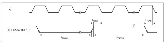
Figure 24.14 TPU Clock Input Timing
