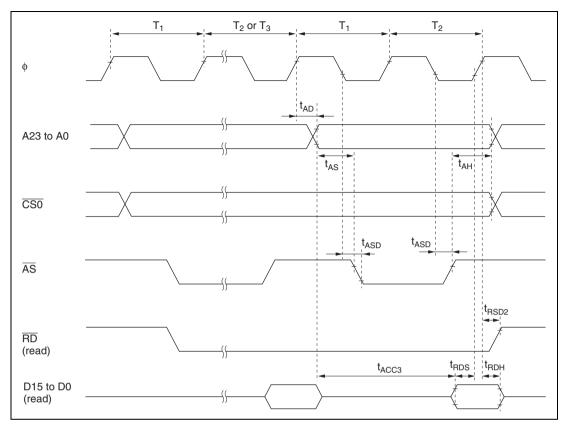
Figure 25.10 Burst ROM Access Timing (Two-State Access)
