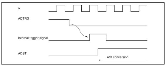
Figure 16.6 External Trigger Input Timing
