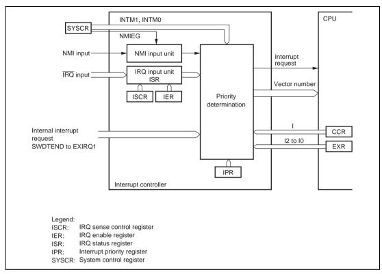
Figure 5.1 Block Diagram of Interrupt Controller
