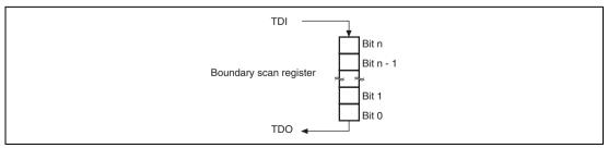
Figure 14.5 Serial Data Input/Output
