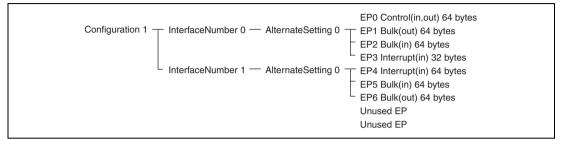
Figure 15.29 Endpoint Configuration Example
