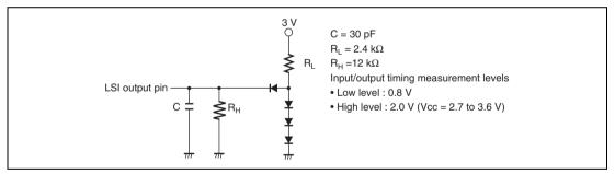
Figure 24.2 Output Load Circuit
