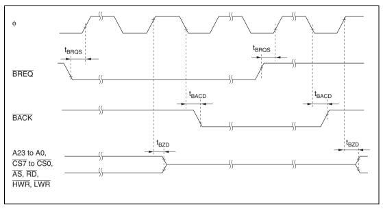
Figure 25.11 External Bus Release Timing
