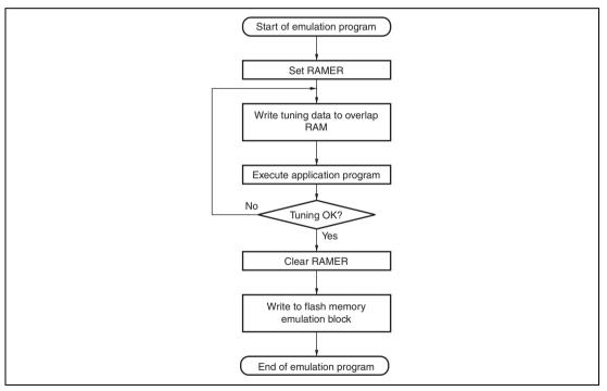
Figure 19.9 Flowchart for Flash Memory Emulation in RAM
