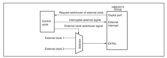
Figure 21.13 Example of External Clock Switching Circuit
