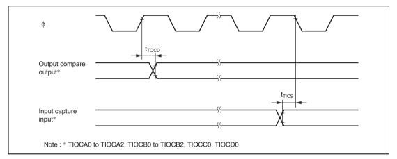
Figure 25.13 TPU Input/Output Timing
