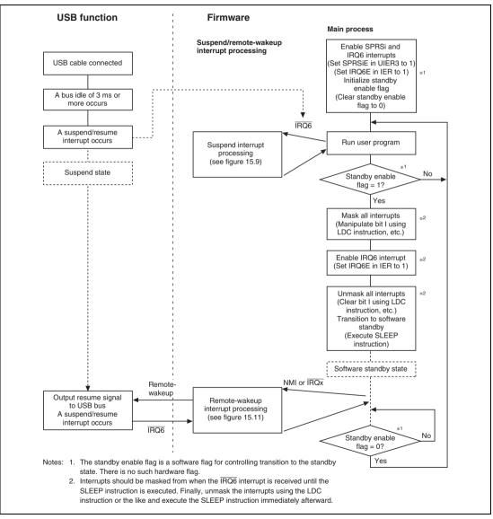
Figure 15.10 Example Flowchart of Suspend and Remote-Wakeup Operations
