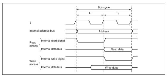
Figure 6.6 On-Chip Peripheral Module Access Cycle
