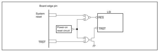
Figure 14.4 Recommended Reset Signal Design
