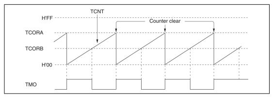
Figure 11.2 Example of Pulse Output
