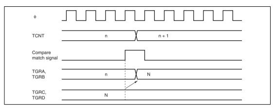
Figure 10.36 Buffer Operation Timing (Compare Match)
