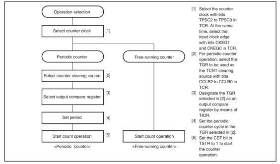
Figure 10.6 Example of Counter Operation Setting Procedure
