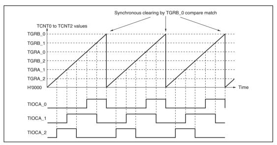
Figure 10.15 Example of Synchronous Operation
