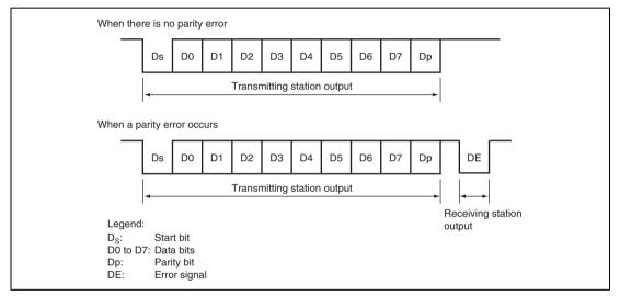
Figure 13.26 Normal Smart Card Interface Data Format
