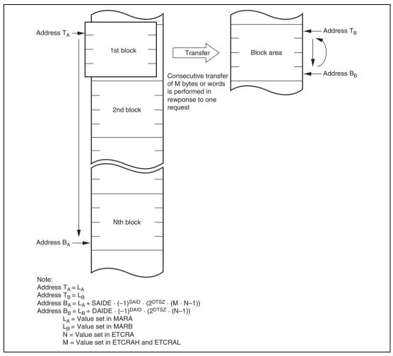
Figure 7.11 illustrates operation in block transfer mode when MARB is designated as a block area.
