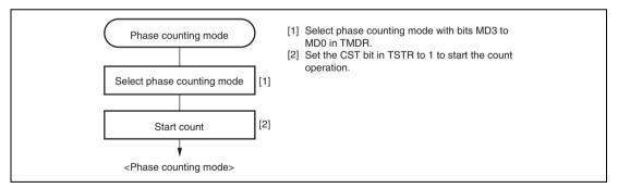
Figure 10.25 Example of Phase Counting Mode Setting Procedure
