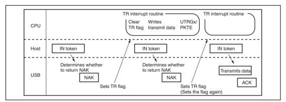
Figure 15.38 TR Interrupt Flag Set Timing
