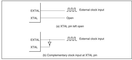
Figure 21.5 External Clock Input (Examples)
