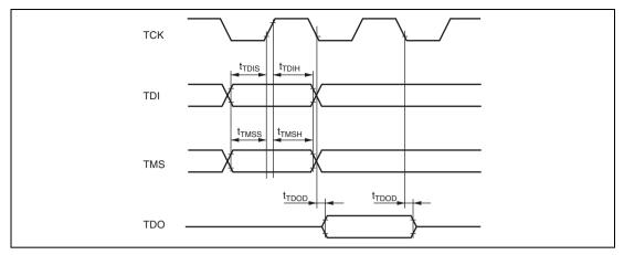
Figure 27.23 Boundary Scan Data Transmission Timing
