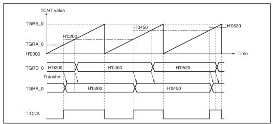
Figure 10.19 Example of Buffer Operation (1)
