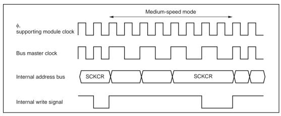
Figure 22.2 Medium-Speed Mode Transition and Clearance Timing
