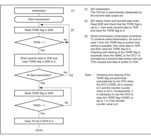
Figure 13.21 Sample Serial Transmission Data Flowchart
