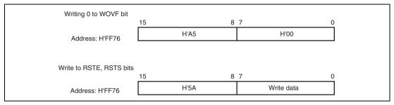
Figure 12.7 Format of Data Written to RSTCSR (Example of WDT0)
