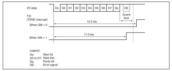
Figure 13.31 TEND Flag Generation Timing in Transmission Operation
