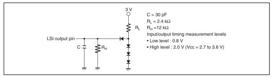
Figure 27.2 Output Load Circuit
