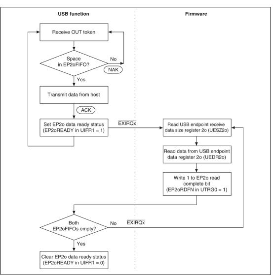
Figure 15.20 EP2o Bulk-Out Transfer Operation
