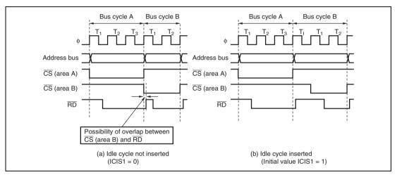
In the initial state after reset release, idle cycle insertion (b) is set.
