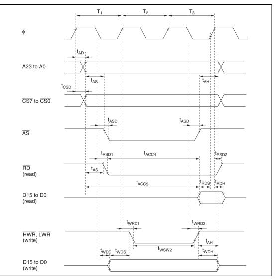
Figure 24.8 Basic Bus Timing (Three-State Access)
