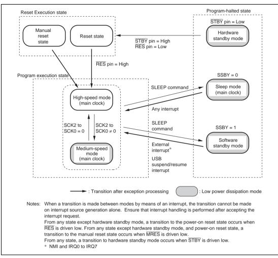
Figure 22.1 Mode Transition Diagram
