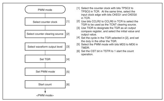
Figure 10.21 Example of PWM Mode Setting Procedure
