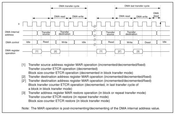
Figure 7.26 DMAC Register Update Timing
