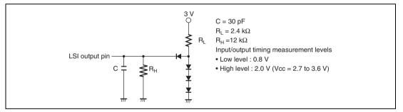
Figure 25.2 Output Load Circuit
