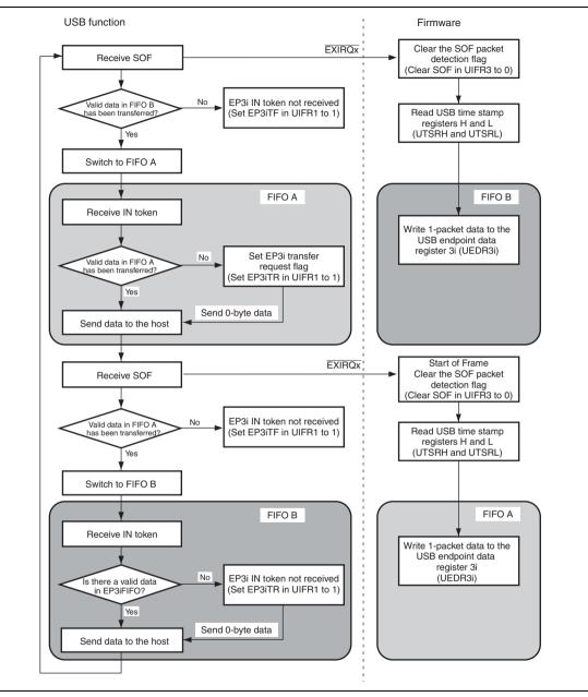
Figure 15.21 EP3i Isochronous-In Transfer Operation
