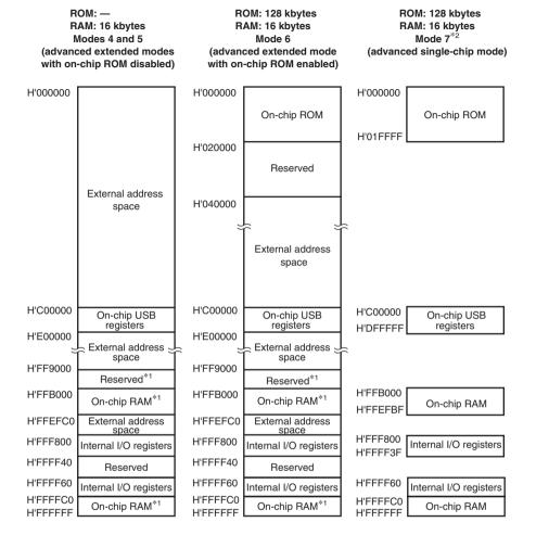
Notes: 1. External addresses can be accessed by clearing the RAME bit in SYSCR to 0.
