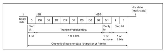
Figure 13.6 Data Format in Asynchronous Communication (Example with 8-Bit Data, Parity, Two Stop Bits)
