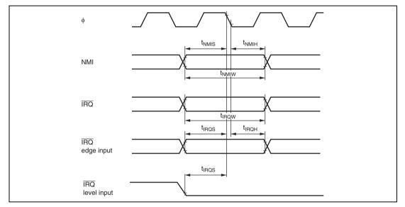
Figure 27.6 Interrupt Input Timing
