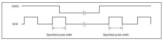
Figure 13.35 Timing for Fixing Clock Output Level
