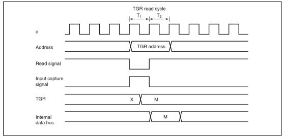
Figure 10.49 Contention between TGR Read and Input Capture
