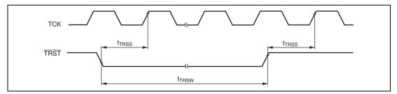
Figure 25.22 Boundary Scan TRST Input Timing (At Reset Hold)
