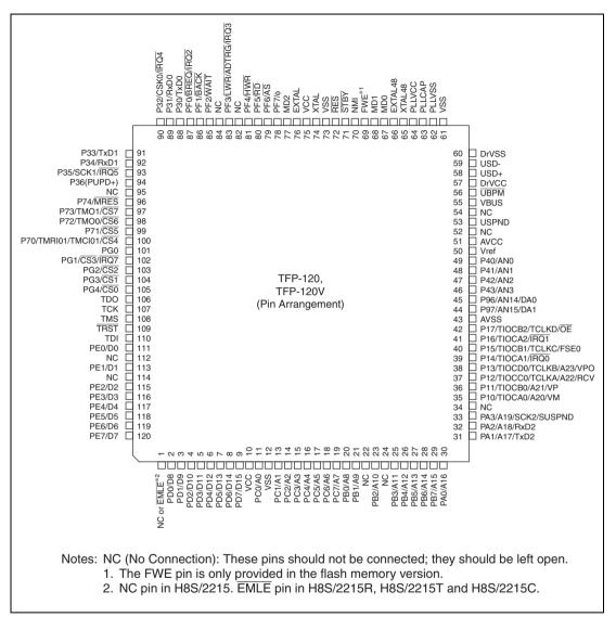
Figure 1.2 Pin Arrangement (TFP-120, TFP-120V)
