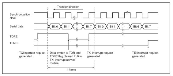
Figure 13.20 Sample SCI Transmission Operation in Clocked Synchronous Mode
