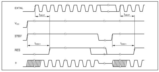
Figure 26.4 Oscillation Stabilization Timing
