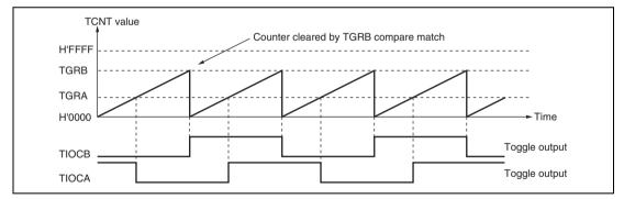
Figure 10.11 Example of Toggle Output Operation
