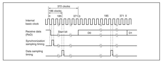
Figure 13.29 Receive Data Sampling Timing in Smart Card Mode (Using Clock of 372 Times the Transfer Rate)
