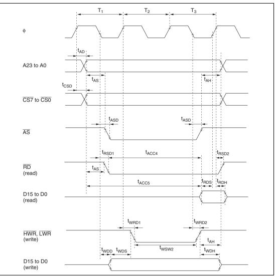
Figure 25.8 Basic Bus Timing (Three-State Access)
