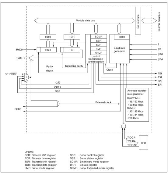
Figure 13.1 Block Diagram of SCI\_0 (H8S/2215)
