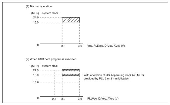
Figure 27.1 Power Supply Voltage and Operating Ranges
