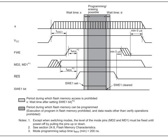
Figure 19.14 Power-On/Off Timing (Boot Mode)
