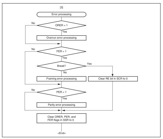
Figure 13.13 Sample Serial Reception Data Flowchart (2)
