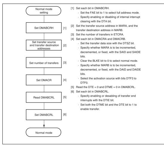
Figure 7.10 Example of Normal Mode Setting Procedure
