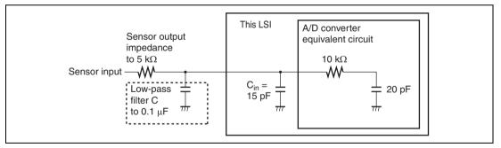
Figure 16.9 Example of Analog Input Circuit
