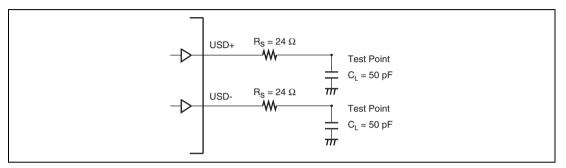
Figure 25.25 Test Load Circuit
