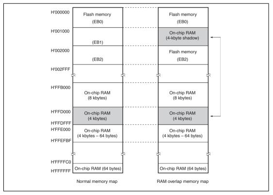
Figure 19.10 Example of RAM Overlap Operation
