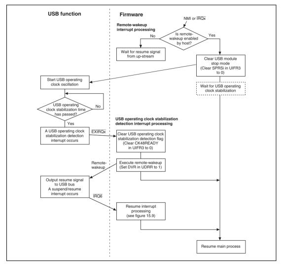
Figure 15.11 Example Flowchart of Remote-Wakeup Interrupt Processing
