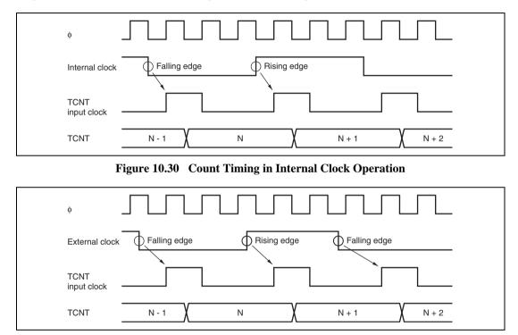
Figure 10.31 Count Timing in External Clock Operation
