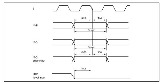
Figure 26.6 Interrupt Input Timing
