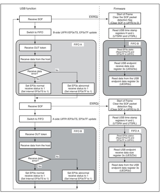
Figure 15.22 EP3o Isochronous-Out Transfer Operation
