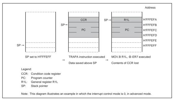
Figure 4.4 Operation when SP Value Is Odd
