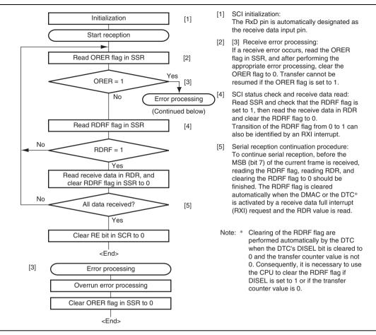
Figure 13.23 Sample Serial Reception Flowchart
