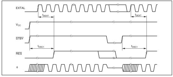
Figure 24.4 Oscillation Stabilization Timing
