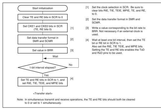
Figure 13.19 Sample SCI Initialization Flowchart
