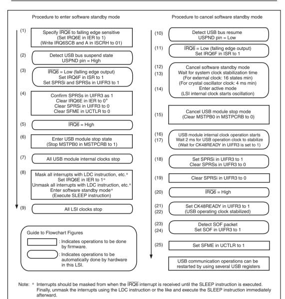
Figure 15.36 Transition to and from Software Standby Mode
