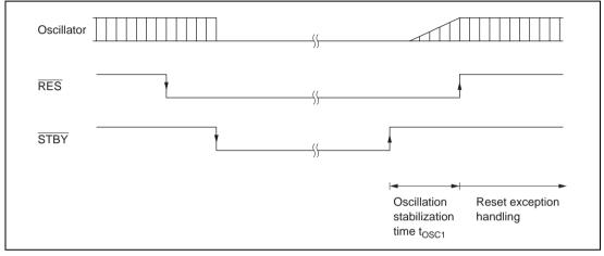
Figure 22.4 Hardware Standby Mode Timing (Example)
