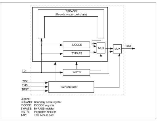
Figure 14.1 Block Diagram of Boundary Scan Function
