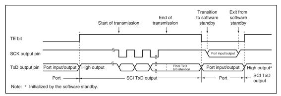
Figure 13.42 Port Pin State of Synchronous Transmission Using Internal Clock
