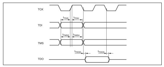
Figure 26.23 Boundary Scan Data Transmission Timing
