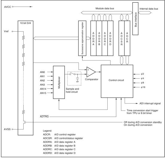
Figure 16.1 Block Diagram of A/D Converter
