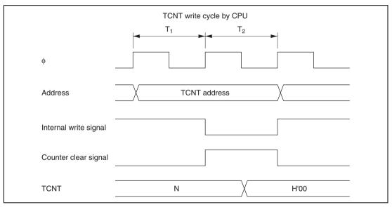
Figure 11.10 Contention between TCNT Write and Clear
