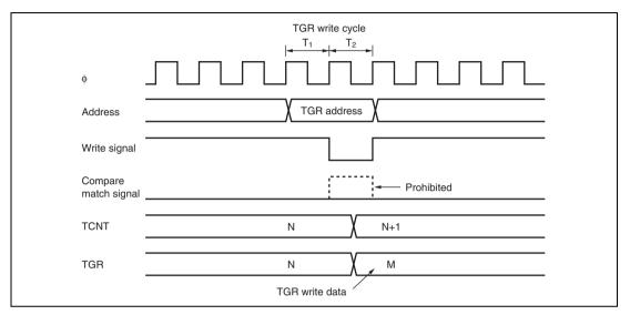
Figure 10.47 Contention between TGR Write and Compare Match
