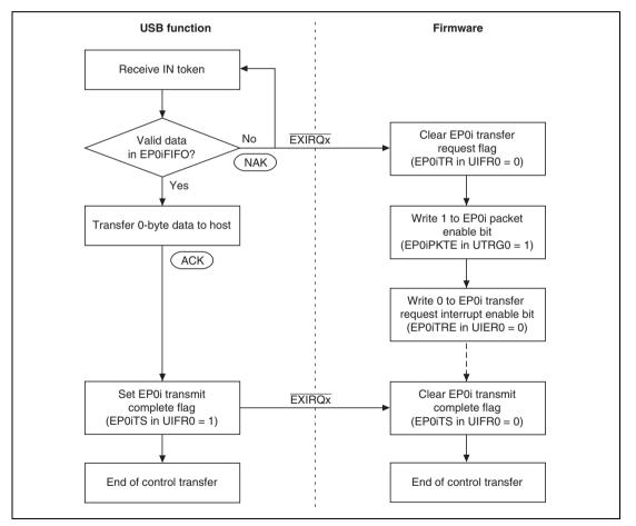
Figure 15.17 Status Stage Operation (Control-Out)
