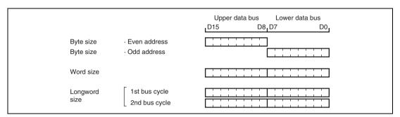
Figure 6.9 Access Sizes and Data Alignment Control (16-Bit Access Space)
