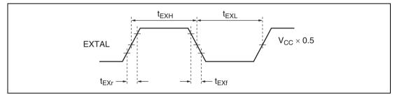
Figure 21.6 External Clock Input Timing
