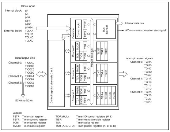
Figure 10.1 Block Diagram of TPU
