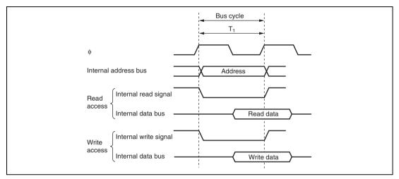
Figure 6.4 On-Chip Memory Access Cycle
