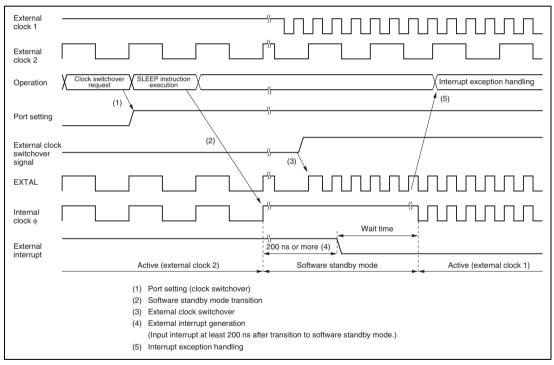
Figure 21.14 Example of External Clock Switchover Timing
