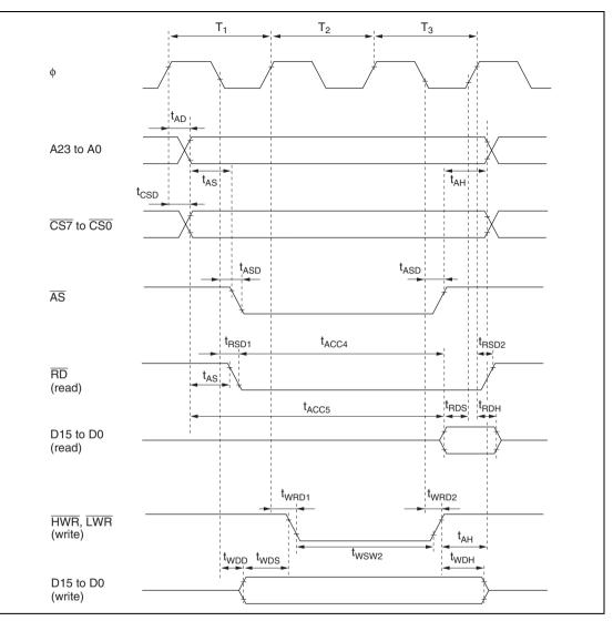
Figure 27.8 Basic Bus Timing (Three-State Access)
