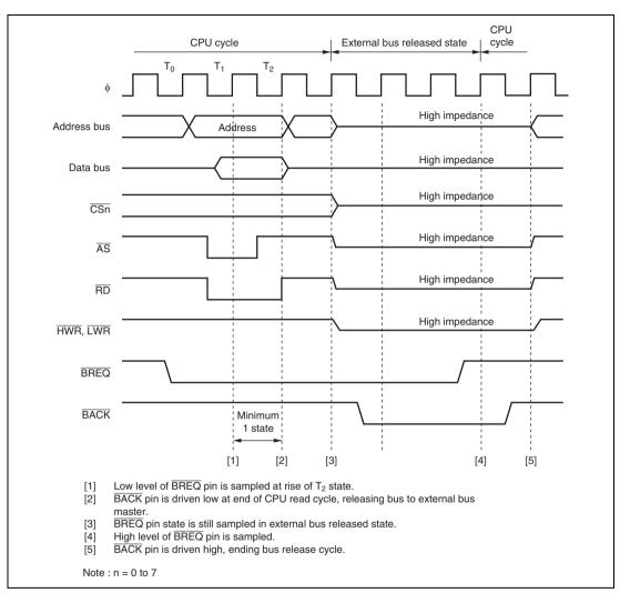
Figure 6.25 shows the timing for transition to the bus-released state.
