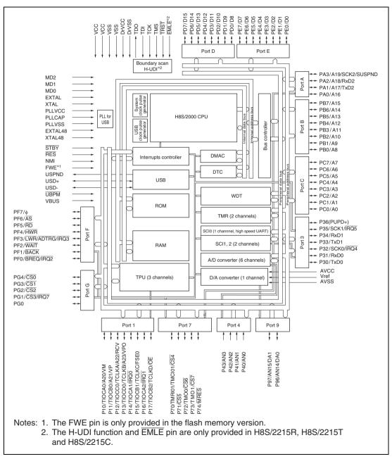
Figure 1.1 Internal Block Diagram
