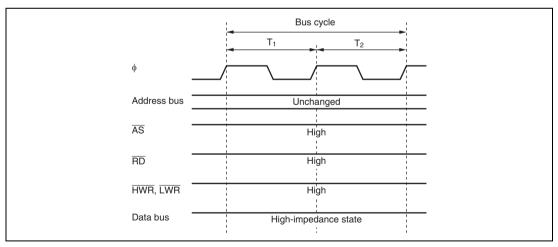
Figure 6.7 Pin States during On-Chip Peripheral Module Access
