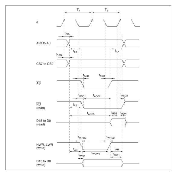
Figure 27.7 Basic Bus Timing (Two-State Access)
