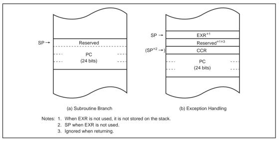
Figure 2.4 Stack Structure in Advanced Mode
