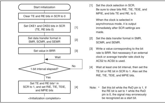
Figure 13.9 Sample SCI Initialization Flowchart
