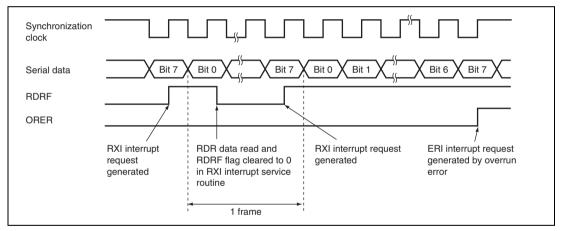
Figure 13.22 Example of SCI Operation in Reception
