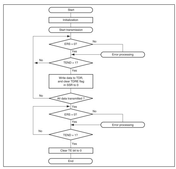
Figure 13.32 Example of Transmission Processing Flow
