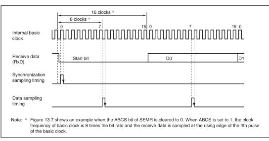
Figure 13.7 Receive Data Sampling Timing in Asynchronous Mode
