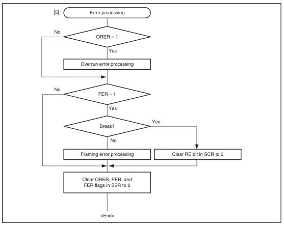
Figure 13.17 Sample Multiprocessor Serial Reception Flowchart (2)
