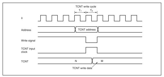
Figure 10.46 Contention between TCNT Write and Increment Operations
