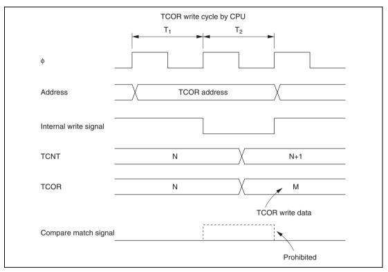
Figure 11.12 Contention between TCOR Write and Compare Match
