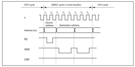
Figure 7.15 Example of DMA Transfer Bus Timing
