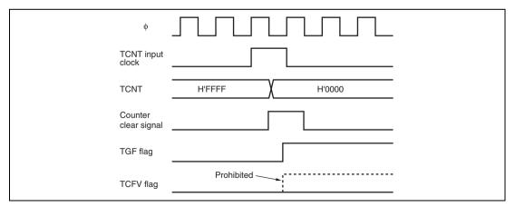
Figure 10.52 Contention between Overflow and Counter Clearing
