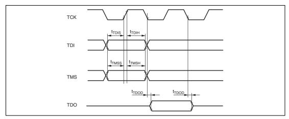
Figure 25.23 Boundary Scan Data Transmission Timing
