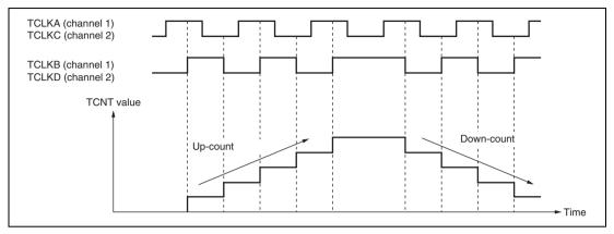
Figure 10.29 Example of Phase Counting Mode 4 Operation
