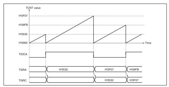
Figure 10.20 Example of Buffer Operation (2)
