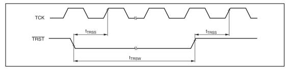
Figure 26.22 Boundary Scan TRST Input Timing (At Reset Hold)
