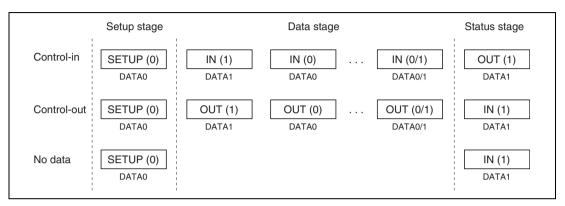
Figure 15.12 Control Transfer Stage Configuration
