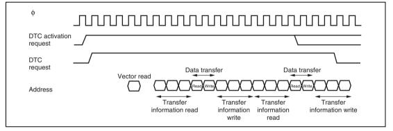
Figure 8.12 DTC Operation Timing (Example of Chain Transfer)
