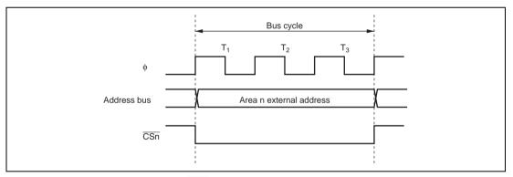
Figure 6.3  $\overline{\text{CSn}}$  Signal Output Timing (n = 0 to 7)
