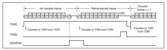
Figure 13.30 Retransfer Operation in SCI Transmit Mode
