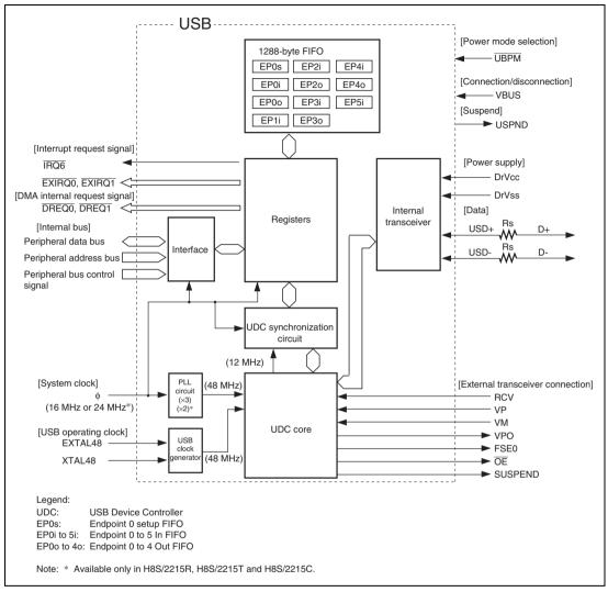
Figure 15.1 Block Diagram of USB
