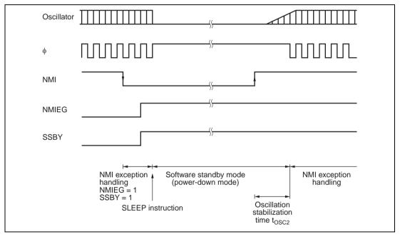
Figure 22.3 Software Standby Mode Application Example
