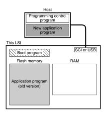
Flash memory initialization The erase program in the boot program area (in RAM) is executed, and the flash memory is initialized (to H'FF). In boot mode, total flash memory erasure is performed, without regard to
