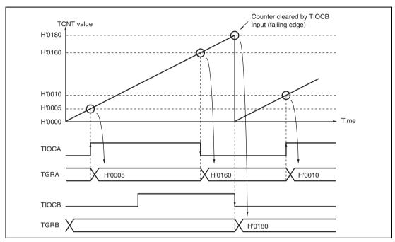
Figure 10.13 Example of Input Capture Operation
