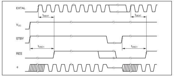
Figure 25.4 Oscillation Stabilization Timing
