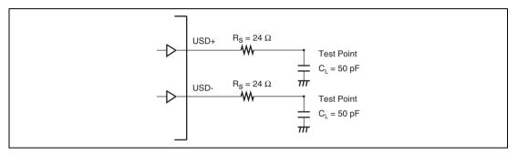
Figure 27.25 Test Load Circuit
