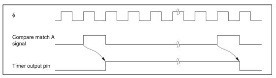
Figure 11.6 Timing of Timer Output
