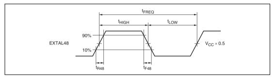
Figure 21.9 48-MHz External Clock Input Timing
