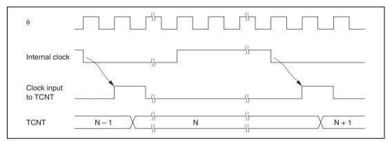
Figure 11.3 Count Timing for Internal Clock Input
