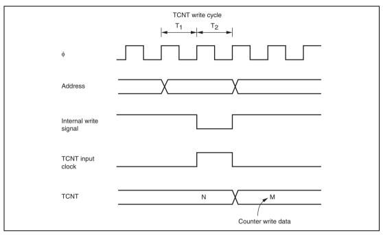
Figure 12.8 Contention between TCNT Write and Increment
