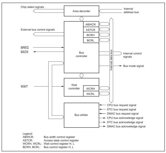
Figure 6.1 Block Diagram of Bus Controller
