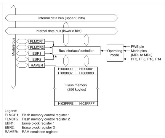
Figure 19.1 Block Diagram of Flash Memory
