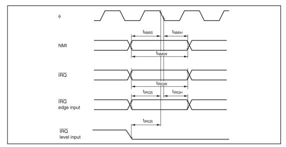
Figure 24.6 Interrupt Input Timing
