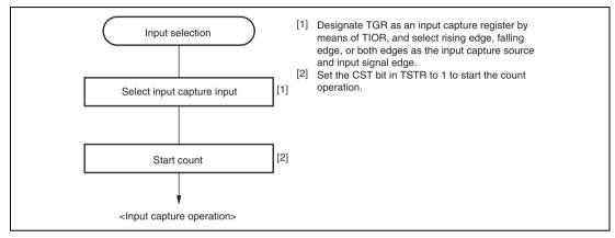
Figure 10.12 Example of Input Capture Operation Setting Procedure
