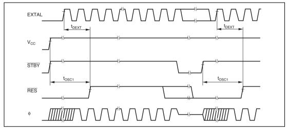
Figure 27.4 Oscillation Stabilization Timing
