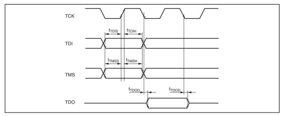
Figure 24.23 Boundary Scan Data Transmission Timing
