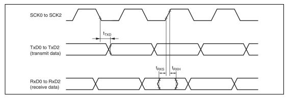
Figure 25.19 SCI Input/Output Timing (Clock Synchronous Mode)
