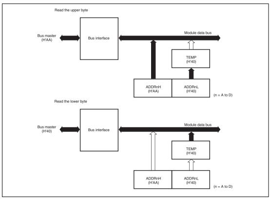
Figure 16.2 Access to ADDR (When Reading H'AA40)
