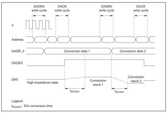
Figure 17.2 Example of D/A Converter Operation
