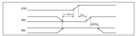
Figure 22.6 Timing of Recovery from Hardware Standby Mode
