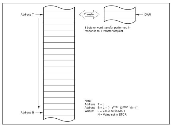
Figure 7.3 Operation in Sequential Mode
