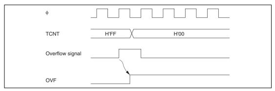
Figure 11.9 Timing of OVF Setting
