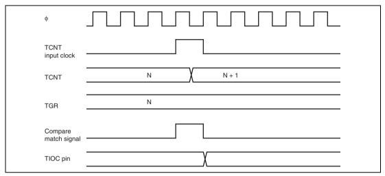
Figure 10.32 Output Compare Output Timing
