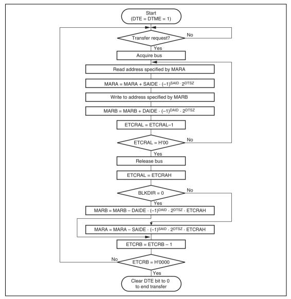
Figure 7.13 Operation Flow in Block Transfer Mode
