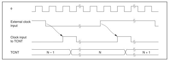
Figure 11.4 Count Timing for External Clock Input
