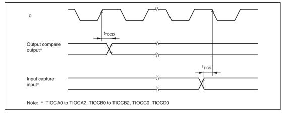
Figure 24.13 TPU Input/Output Timing
