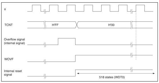
Figure 12.3 Timing of WOVF Setting
