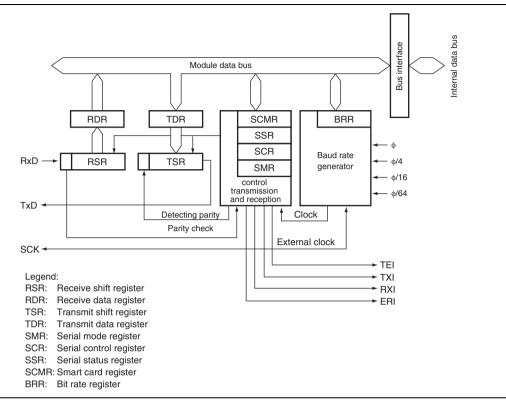
Figure 13.3 Block Diagram of SCI\_1 and SCI\_2
