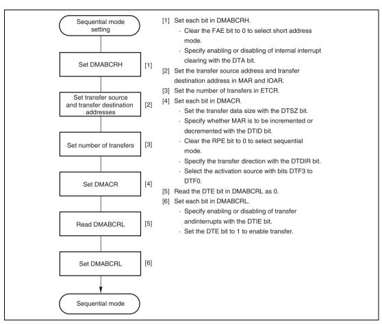
Figure 7.4 Example of Sequential Mode Setting Procedure
