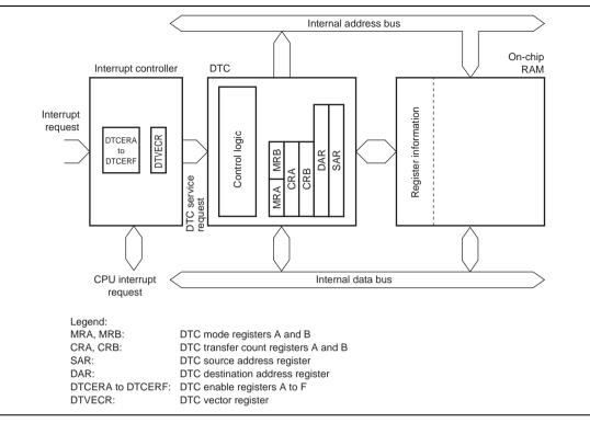
Figure 8.1 Block Diagram of DTC
