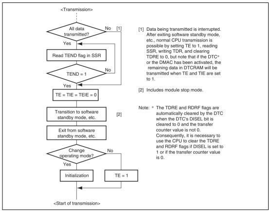
Figure 13.40 Sample Flowchart for Mode Transition during Transmission
