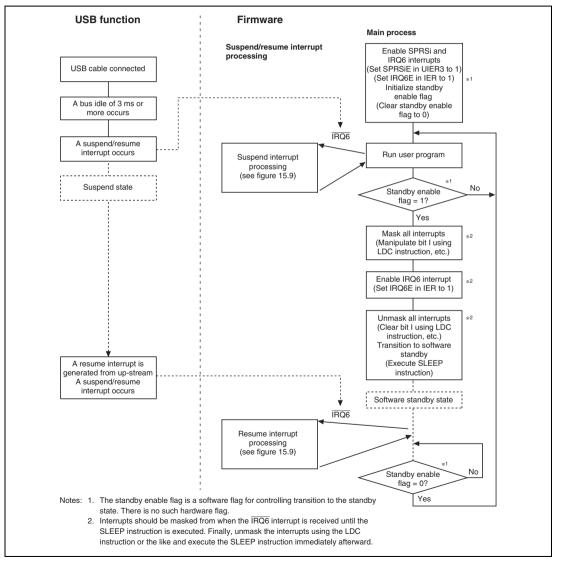
Figure 15.8 Example Flowchart of Suspend and Resume Operations
