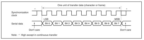
Figure 13.18 Data Format in Synchronous Communication (For LSB-First)
