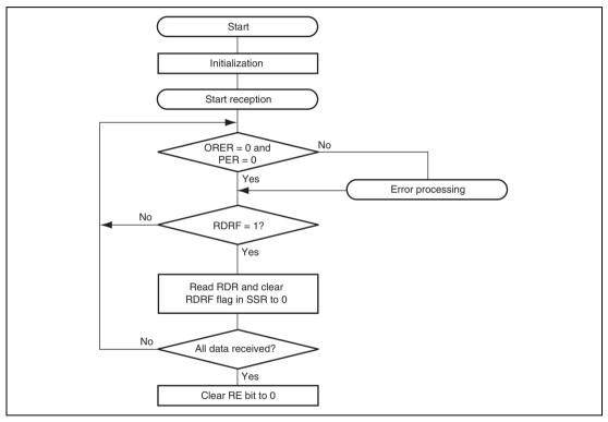
Figure 13.34 Example of Reception Processing Flow
