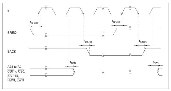
Figure 26.11 External Bus Release Timing
