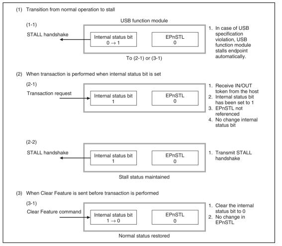
Figure 15.24 Automatic Stall by USB Function Module
