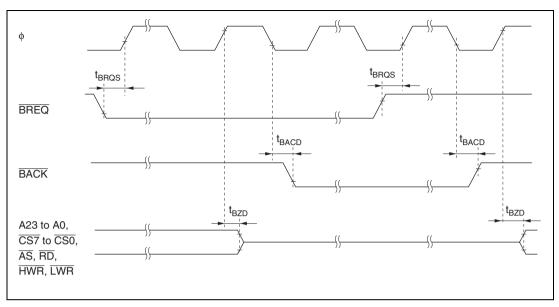
Figure 27.11 External Bus Release Timing
