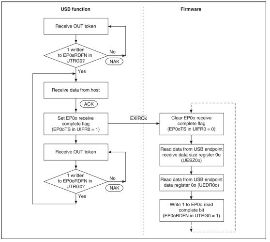
Figure 15.15 Data Stage Operation (Control-Out)
