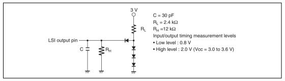
Figure 26.2 Output Load Circuit
