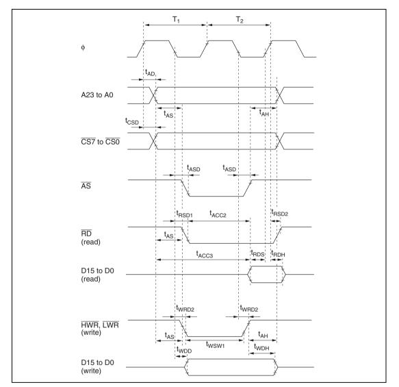
Figure 25.7 Basic Bus Timing (Two-State Access)
