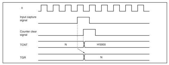
Figure 10.35 Counter Clear Timing (Input Capture)
