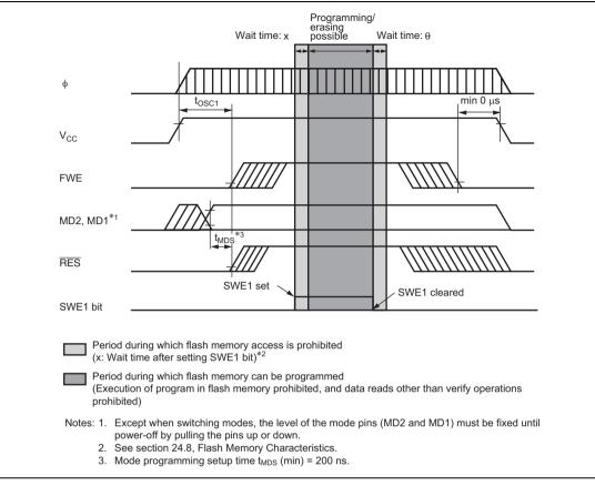
Figure 19.15 Power-On/Off Timing (User Program Mode)
