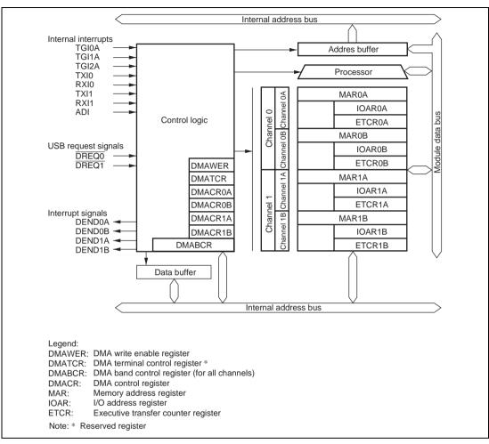
Figure 7.1 Block Diagram of DMAC
