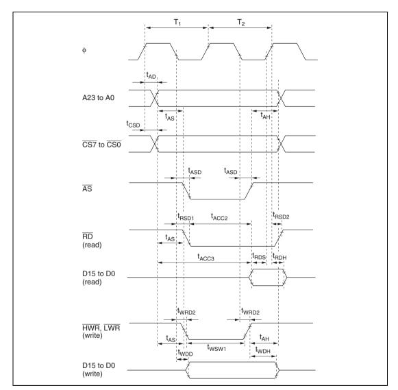
Figure 24.7 Basic Bus Timing (Two-State Access)
