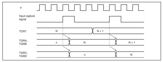
Figure 10.37 Buffer Operation Timing (Input Capture)
