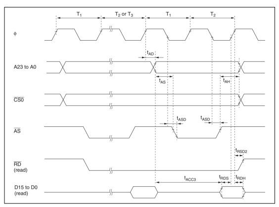
Figure 26.10 Burst ROM Access Timing (Two-State Access)
