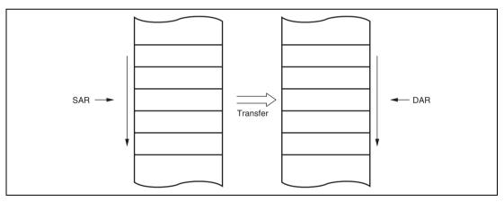
Figure 8.6 Memory Mapping in Normal Mode
