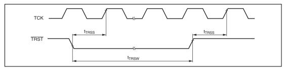
Figure 24.22 Boundary Scan TRST Input Timing (At Reset Hold)
