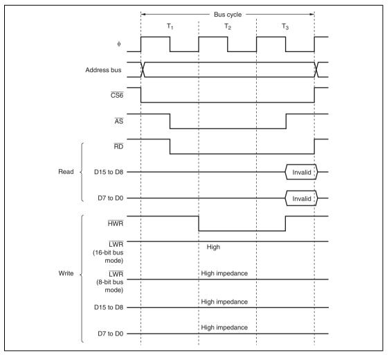
Figure 6.12 Bus Timing for Area 6
