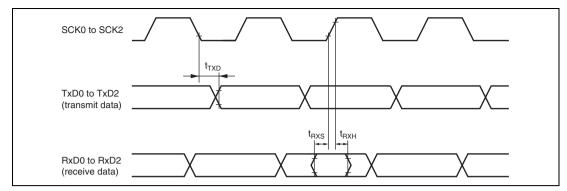
Figure 27.19 SCI Input/Output Timing (Clock Synchronous Mode)
