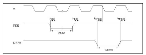
Figure 24.5 Reset Input Timing
