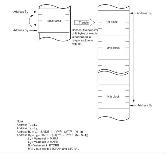
Figure 7.12 Operation in Block Transfer Mode (BLKDIR = 1)
