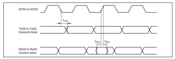
Figure 26.19 SCI Input/Output Timing (Clock Synchronous Mode)
