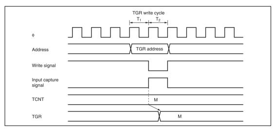
Figure 10.50 Contention between TGR Write and Input Capture
