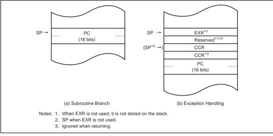
Figure 2.2 Stack Structure in Normal Mode
