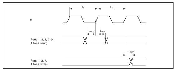
Figure 26.12 I/O Port Input/Output Timing
