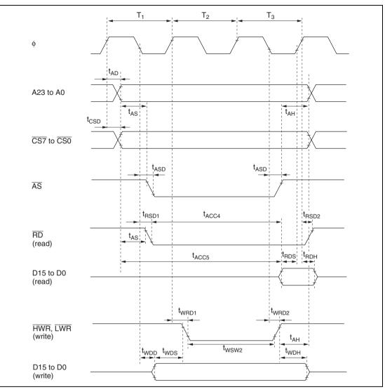
Figure 26.8 Basic Bus Timing (Three-State Access)
