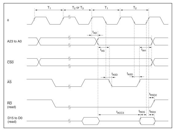
Figure 24.10 Burst ROM Access Timing (Two-State Access)
