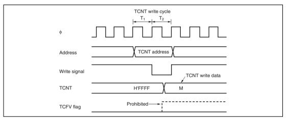
Figure 10.53 Contention between TCNT Write and Overflow
