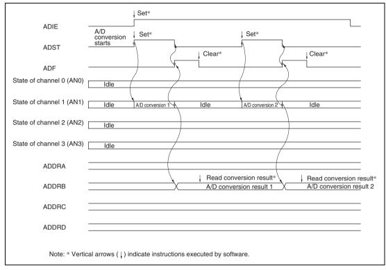
Figure 16.3 A/D Conversion Timing (Single-Chip Mode, Channel 1 Selected)
