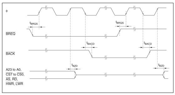
Figure 24.11 External Bus Release Timing
