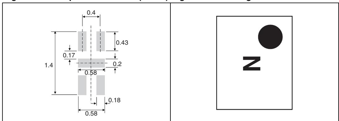
**Note:** Product marking may be rotated by multiples of 90° for assembly plant differentiation. In no case should this product marking be used to orient the component for its placement on a PCB. Only pin 1 mark is to be used for this purpose.
