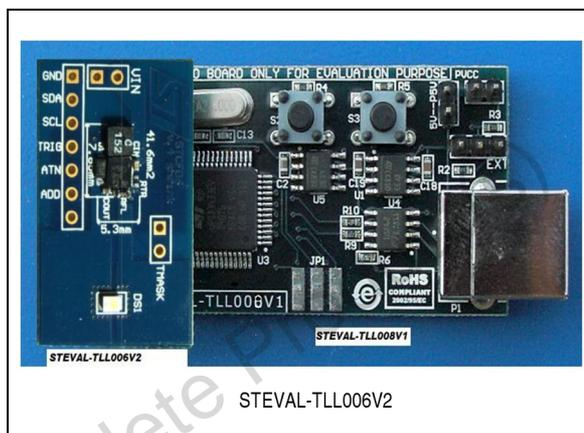
Connect the motherboard to the PC through the USB cable (AB type). Wait until the computer enumerates the control board and displays the message that new hardware has been found and is ready to use. It is then possible to run the data packet creator application by pressing the “Connect board” button.
