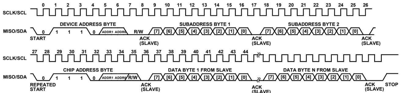
Figure 28. I<sup>2</sup>C Slave Burst Mode Read Operation (N Bytes)
