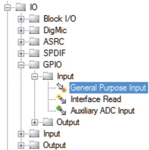
Figure 72. General-Purpose Input in the SigmaStudio Toolbox
