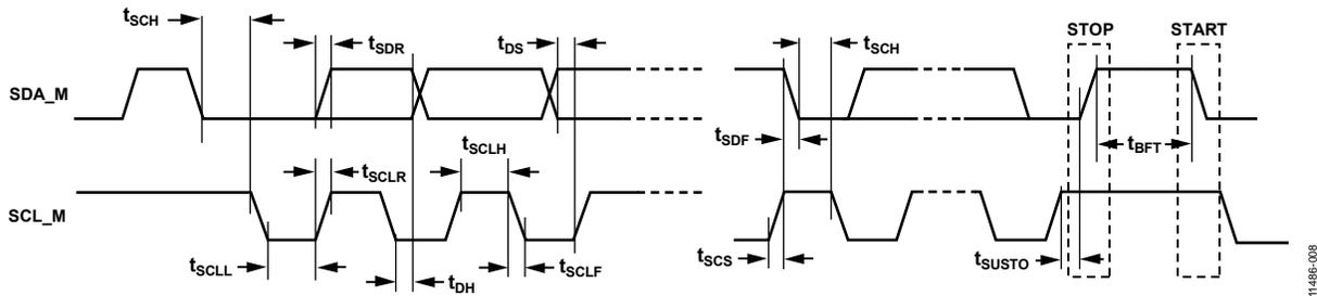
Figure 7. I<sup>2</sup>C Master Port Timing Specifications
