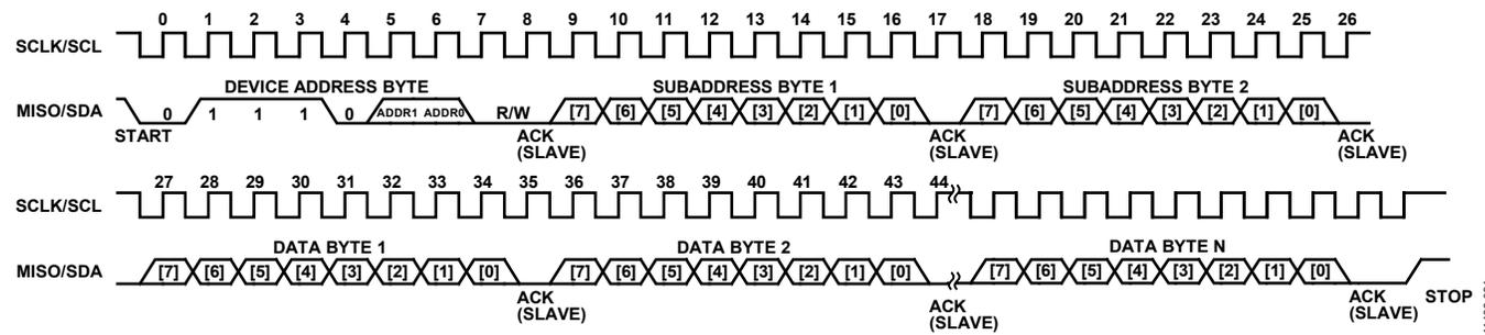
Figure 27. I<sup>2</sup>C Slave Burst Mode Write Operation (N Bytes)
