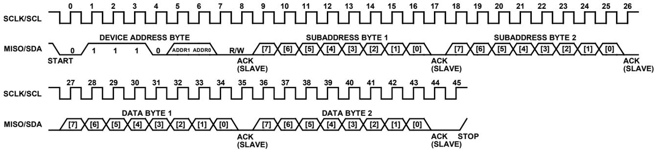
Figure 26. I<sup>2</sup>C Slave Single Word Write Operation (Two Bytes)
