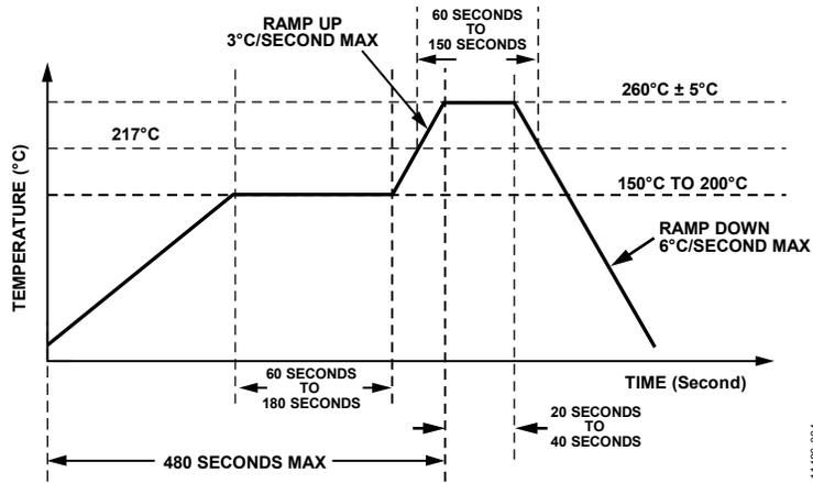
Figure 88. Soldering Profile
