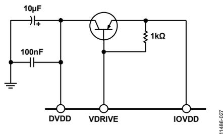
Figure 21. External Components Required for Voltage Regulator Circuit
