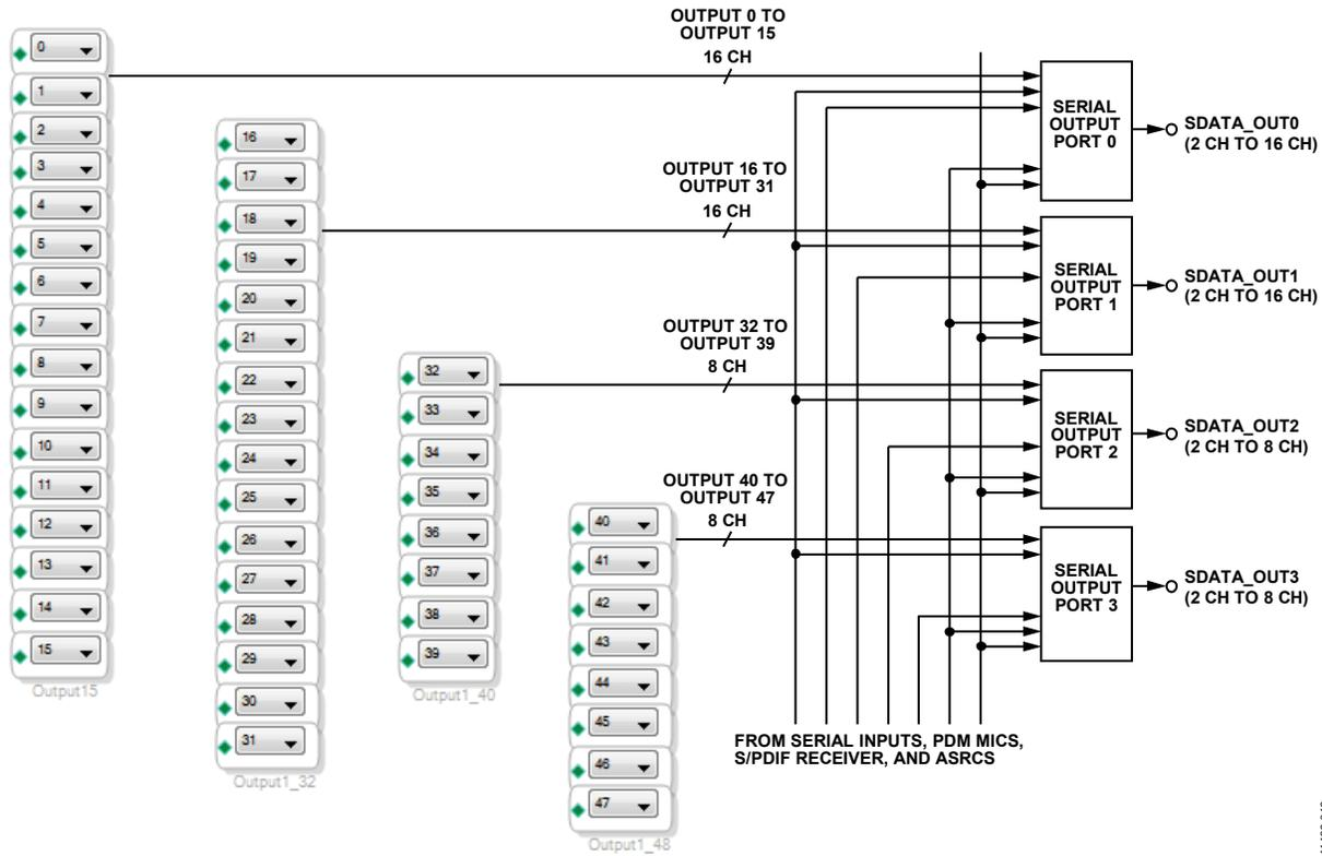
Figure 45. DSP to Serial Output Mapping in SigmaStudio
