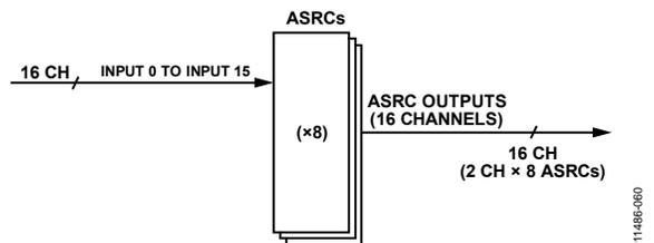
Figure 56. Example ASRC Routing, Bypassing DSP Core
