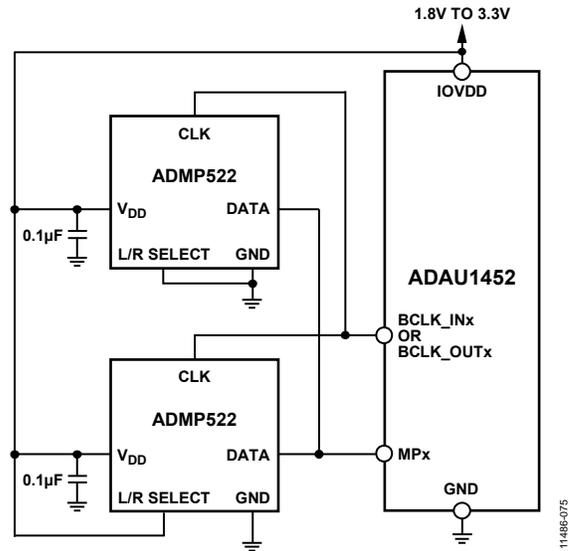
Figure 71. Example Stereo PDM Microphone Input Circuit
