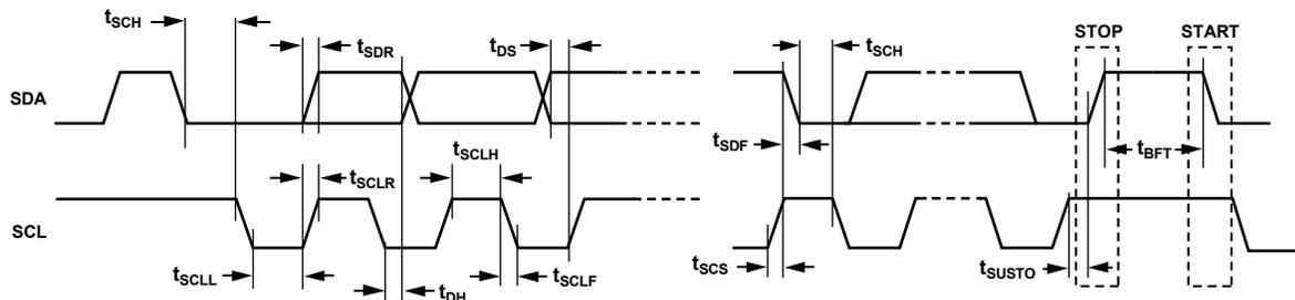
Figure 6. I<sup>2</sup>C Slave Port Timing Specifications
