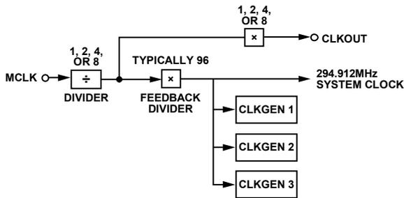
Figure 20. Clock Output Generator
