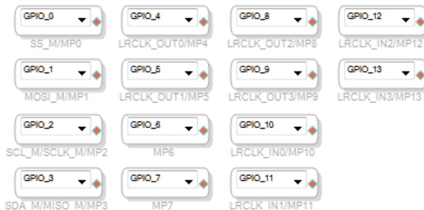
Figure 74. Complete Set of General-Purpose Inputs in SigmaStudio
