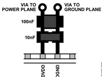
Figure 81. Layout for Multiple Power Supply Bypass Capacitors
