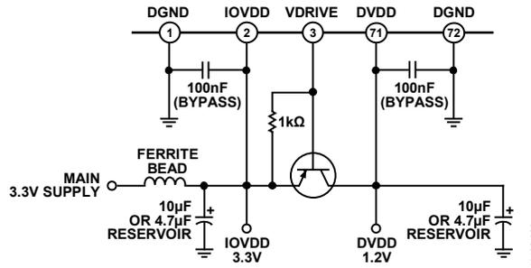
Figure 85. Ferrite Bead Power Supply Isolation Circuit Example
