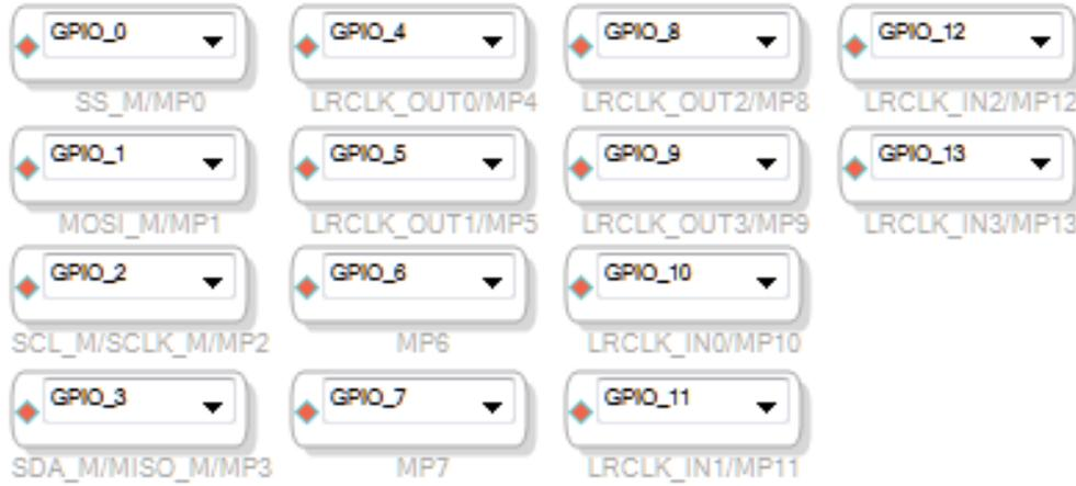
Figure 75. Complete Set of General-Purpose Outputs in SigmaStudio
