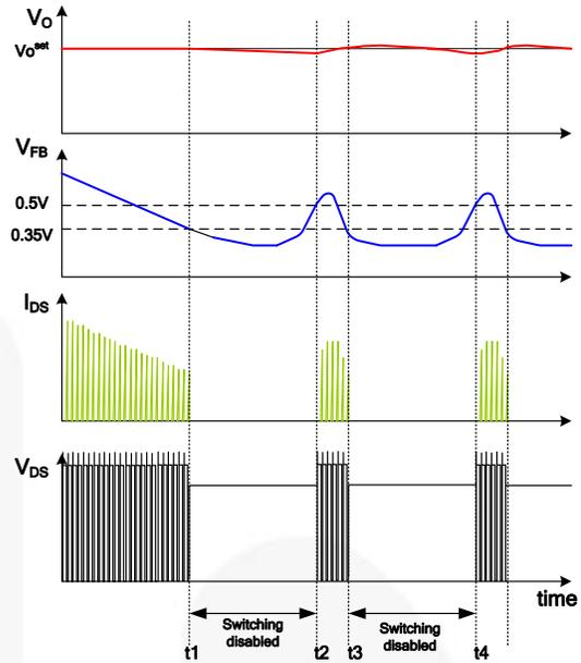
Figure 22. Burst-Mode Operation
