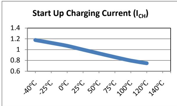
Figure 10. Start Up Charging Current vs. Temperature
