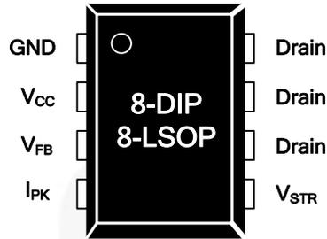
Figure 3. Pin Configuration
