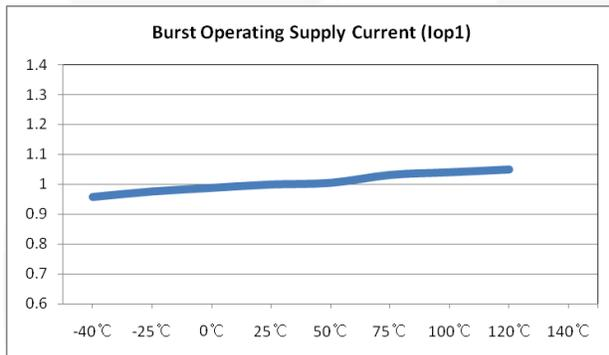
Figure 12. Burst Operating Supply Current vs. Temperature
