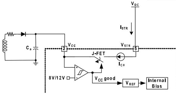
Figure 14. Startup Circuit
