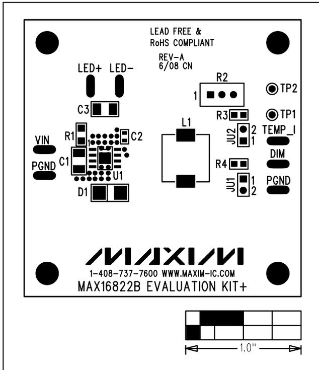
Figure 2. MAX16822B EV Kit Component Placement Guide—Components Side
