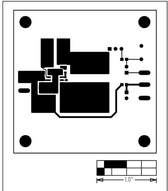
Figure 3. MAX16822B EV Kit PCB Layout—Component Side
