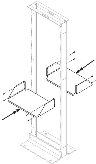
Attach rack mount shelf to the rack at the desired location and secure with provided #12-24 screws. (SRM19CM3 shown)
