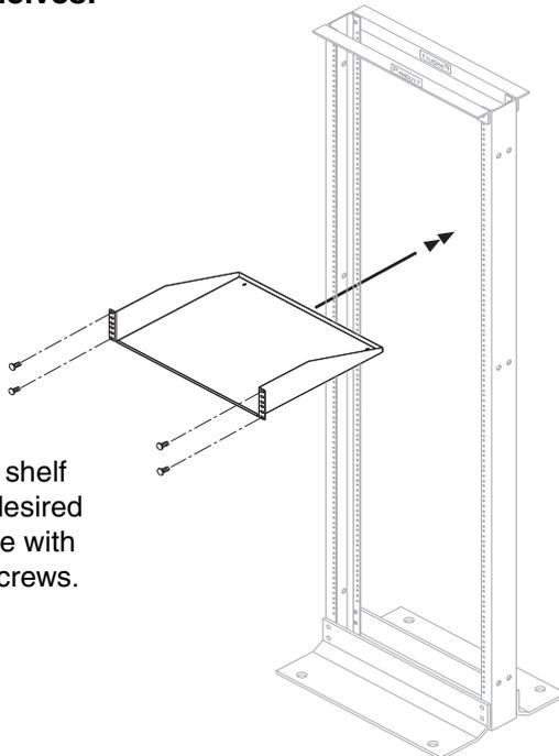
Attach rack mount shelf to the rack at the desired location and secure with provided #12-24 screws.
