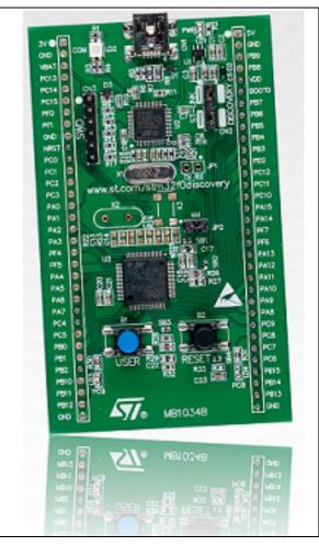
Based on the STM32F051R8T6, it includes an ST-LINK/V2 embedded debug tool, LEDs, pushbuttons and an additional prototyping board for easy connection of additional components and modules.
