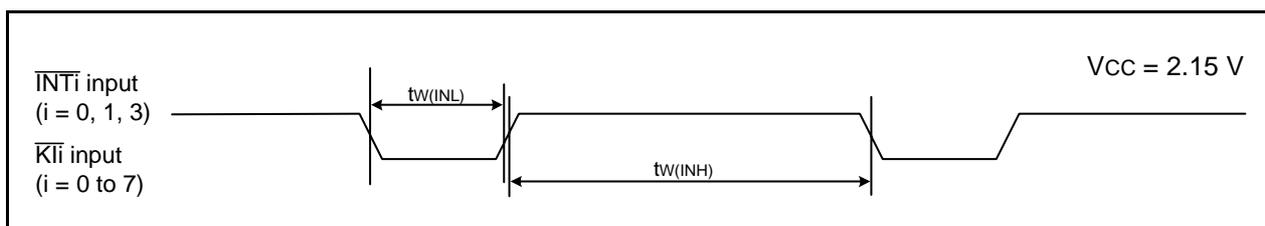
**Figure 5.13 Input Timing Diagram for External Interrupt  $\overline{\text{INT}}_i$  and Key Input Interrupt  $\overline{\text{K}}_i$  when  $V_{CC} = 2.15 \text{ V}$**
