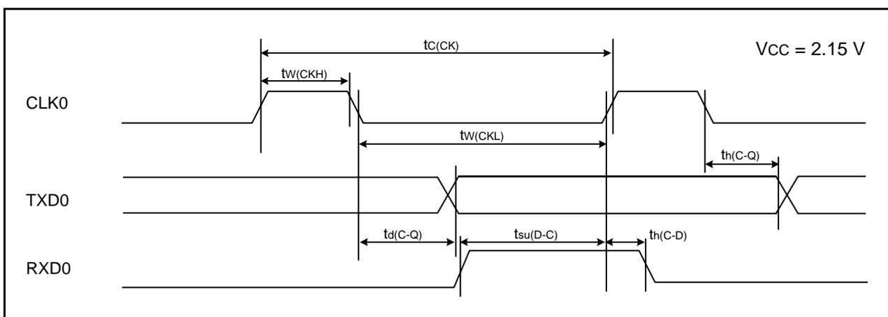
**Figure 5.12** Serial Interface Timing Diagram when  $V_{CC} = 2.15\text{ V}$
