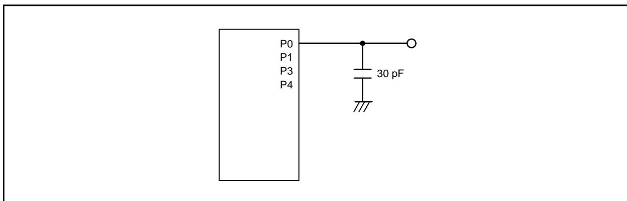
Figure 5.1 Ports P0, P1, P3 and P4 Timing Measurement Circuit
