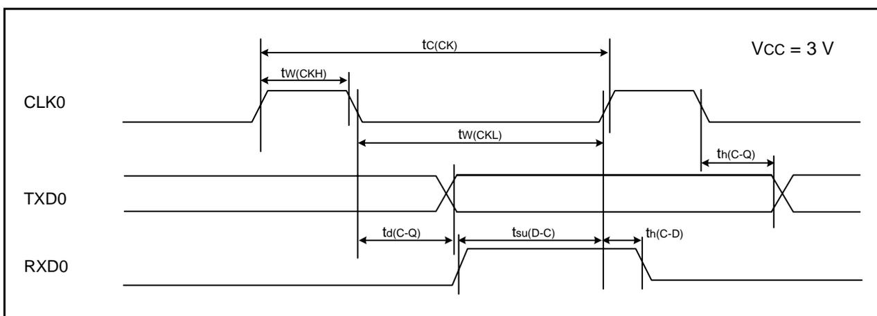
**Figure 5.9 Serial Interface Timing Diagram when Vcc = 3 V**
