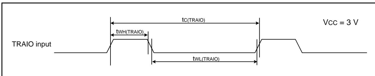
**Figure 5.8 TRAI0 Input Timing Diagram when Vcc = 3 V**
