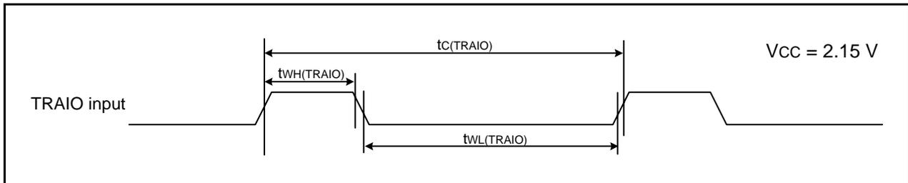
**Figure 5.11** TRAIO Input Timing Diagram when  $V_{CC} = 2.15\text{ V}$ **Table 5.20** Serial Interface
