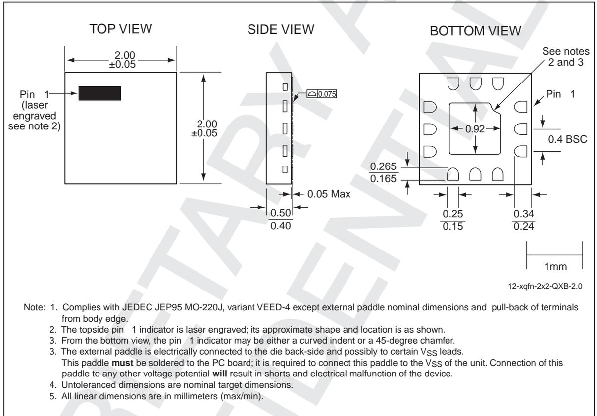
**Figure 12:** 12-Contact Extremely-thin Quad Flat No-lead (XQFN)
