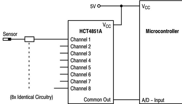
**Figure 8. MC74HCT4851A Solution**
