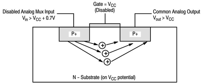
**Figure 20. Diagram of Bipolar Coupling Mechanism**
