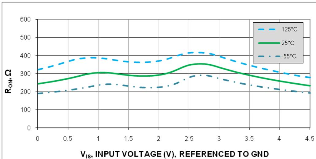
Figure 5. Typical On Resistance V<sub>CC</sub> = 4.5V
