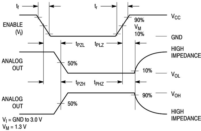
**Figure 17. Propagation Delays, Enable to Analog Out**
