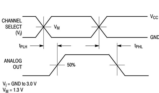
Figure 13. Propagation Delays, Channel Select to Analog Out
