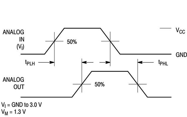
**Figure 15. Propagation Delays, Analog In to Analog Out**
