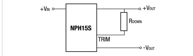
When the output voltage is trimmed up, output current must be derated so that the maximum output power is not exceeded.
