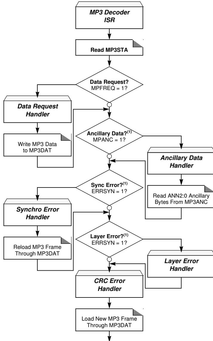
Note: 1. Test these bits only if needed (unmasked interrupt).
