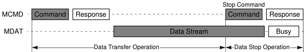
**Figure 18-4.** Multiple Block Write Operation
