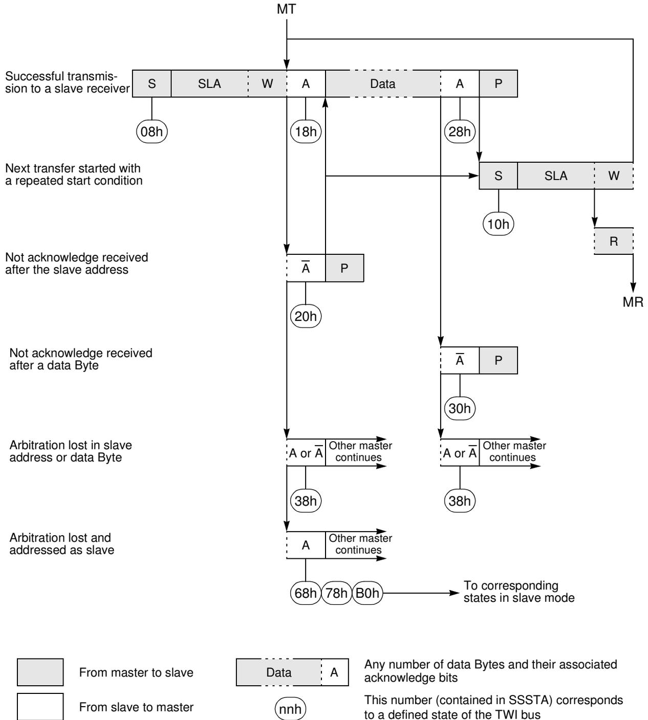
Figure 21-4. Format and States in the Master Receiver Mode
