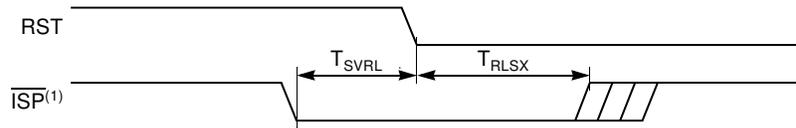
Note: 1.  $\overline{\text{ISP}}$  must be driven through a pull-down resistor (see Section “In System Programming”, page 218).
