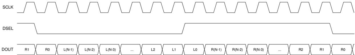
Figure 15-4. 20 bit MSB justified mode
