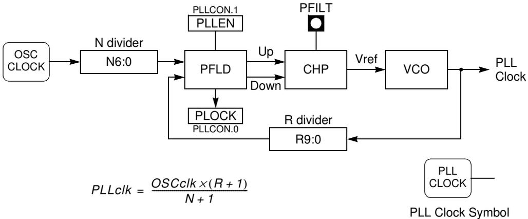
Figure 5-5. PLL Filter Connection
