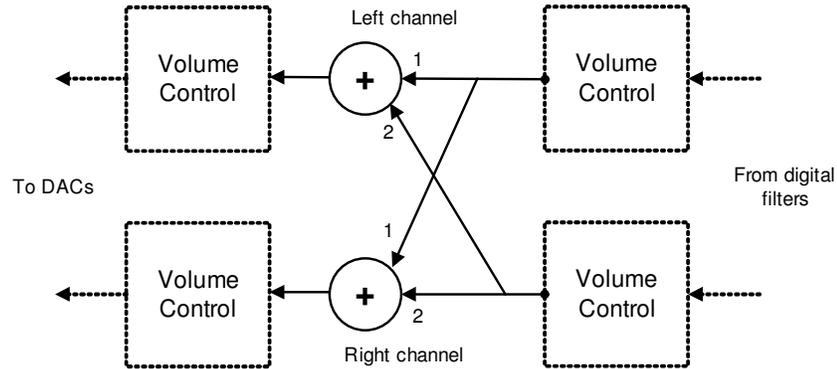
Note: Whenever the two mixer inputs are selected, a  $-6$  dB gain is applied to the output signal. Whenever only one input is selected, no gain is applied.
