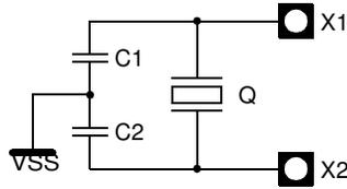
Note: For operation with most standard crystals, no external components are needed on X1 and X2. It may be necessary to add external capacitors on X1 and X2 to ground in special cases (max 10 pF). X1 and X2 may not be used to drive other circuits.
