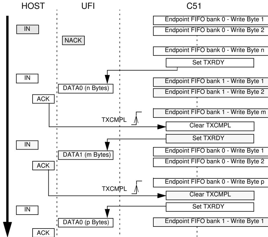
An endpoint should be first enabled and configured before being able to send Bulk or Interrupt packets.
