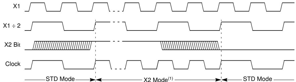
Note: 1. In order to prevent any incorrect operation while operating in X2 mode, user must be aware that all peripherals using clock frequency as time reference (timers, etc.) will have their time reference divided by 2. For example, a free running timer generating an interrupt every 20 ms will then generate an interrupt every 10 ms.
