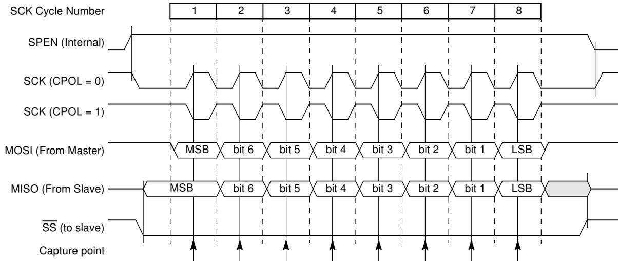
**Figure 19-6.** Data Transmission Format (CPHA = 1)
