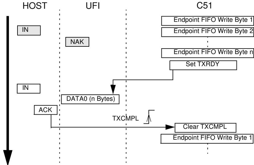
An endpoint should be first enabled and configured before being able to send Bulk or Interrupt packets.
