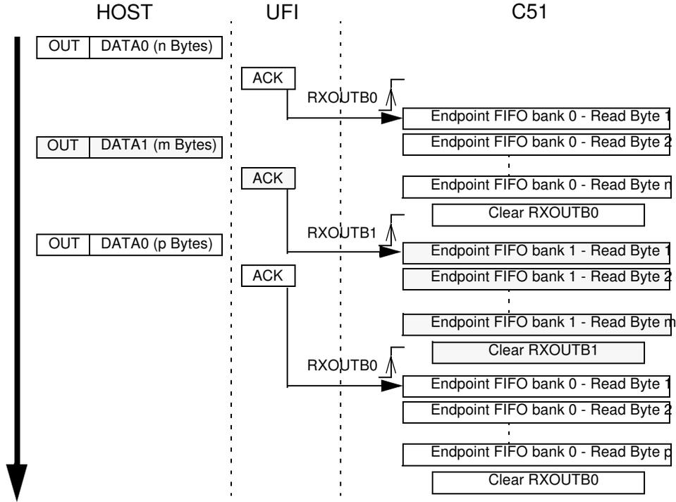
An endpoint should be first enabled and configured before being able to receive Bulk or Interrupt packets.
