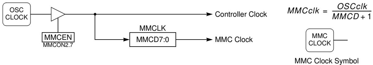
As soon as MMCEN bit in MMCON2 is set, the MMC controller receives its system clock. The MMC command and data clock is generated on MCLK output and sent to the command line and data line controllers. Figure 18-11 shows the MMC controller configuration flow. As exposed in Section "Clock Control", page 139, MMCD7:0 bits can be used to dynamically increase or reduce the MMC clock.
