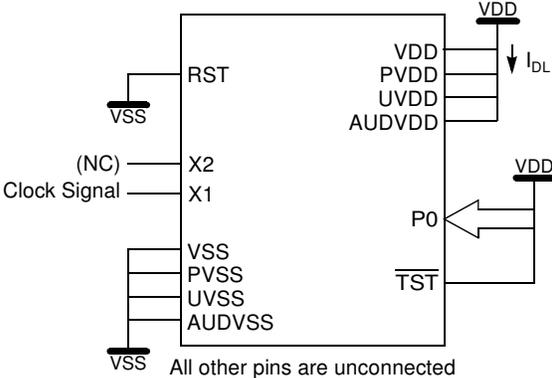
Figure 24-3.  $I_{PD}$  Test Condition, Power-Down Mode
