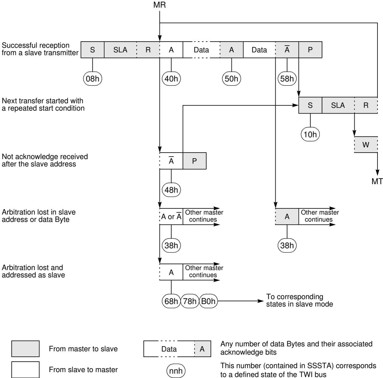
Figure 21-6. Format and States in the Slave Transmitter Mode
