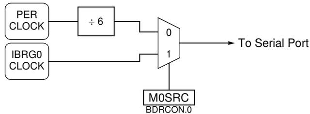
**Figure 20-7.** Baud Rate Formulas (Mode 0)
