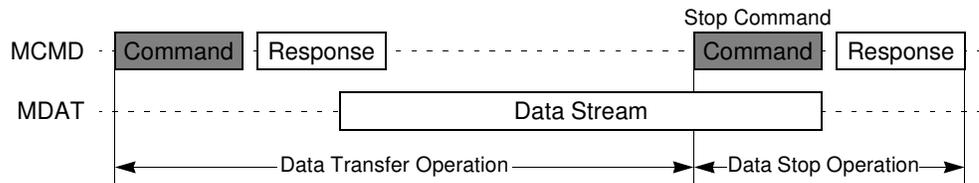
**Figure 18-2.** (Multiple) Block Read Operation
