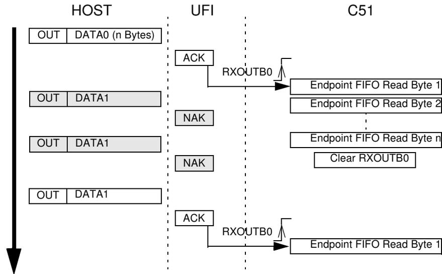
An endpoint should be first enabled and configured before being able to receive Bulk or Interrupt packets.
